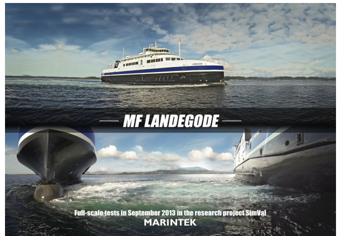
Figure 4. Thruster tests for LNG ferry "Landegode".
