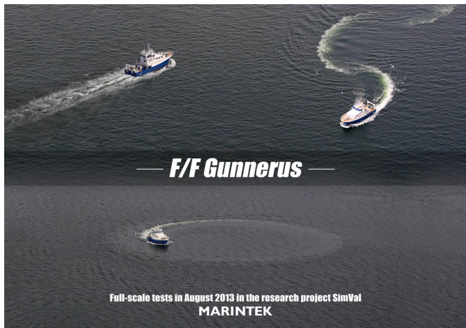
Figure 3. Bird's eye view of some manoeuvring tests for "Gunnerus".
