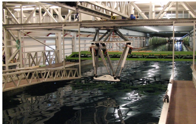
MARINTEK's Hexapod system is mounted on the Seakeeping carriage in the towing tank.
