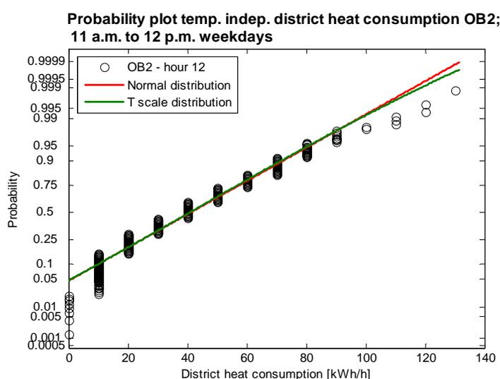
Figure 6.14 Probability plot of temperature-independent district heat consumption for OB2 during hour 11 a.m. to 12 p.m. weekdays, including fitted normal and Student's t distribution.
