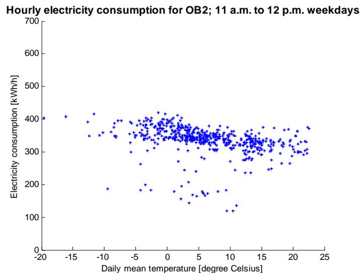
Figure 6.17 Scatter plot of daily mean temperature vs. hourly electricity consumption for OB2 in Trondheim for weekdays during hour 12, i.e. electricity consumption from 11 a.m. to 12 p.m. over a four-year period (2002-2005).
