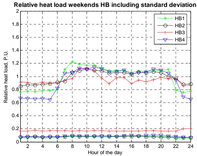
Figure 0.16 Design heat load profiles weekends for all HB analysed.
