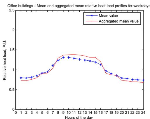
Figure 9 Mean and aggregated mean relative heat load profiles for office buildings weekdays
