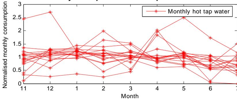
*Figure 4.10 Normalised monthly hot tap water consumption in households with individual hourly measurements of space heating and hot tap water.*
