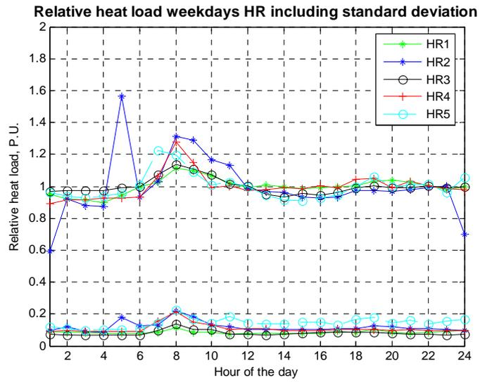
Figure 0.19 Design heat load profiles weekdays for all HR analysed.
