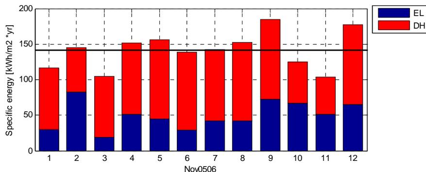
*Figure 7.9 Specific yearly energy consumption for single family houses and apartment blocks plotted for the period from November 1, 2005 until November 1, 2006.*
