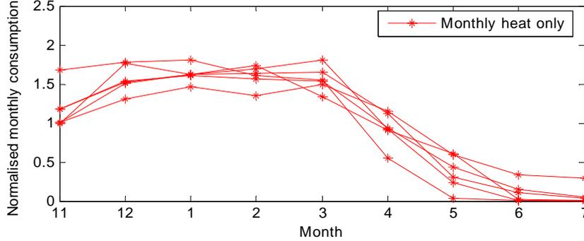
*Figure 4.9 Normalised monthly space heating consumption in households with individual hourly measurements of space heating and hot tap water.*
