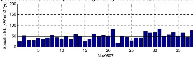
Figure 7.10 Specific yearly district heat and electricity consumption for single family houses and apartment blocks plotted for the period from November 1, 2005 until November 1, 2006. The figure includes 53 buildings with continuous district heat measurements and 38 buildings with continuous electricity measurements.
