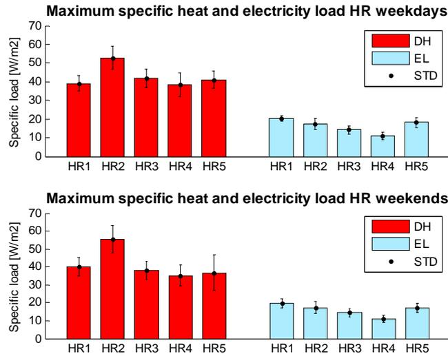
Figure 7.6 Maximum specific heat and electricity load including specific standard deviation intervals for each hotel and restaurant building analysed for both day types.
