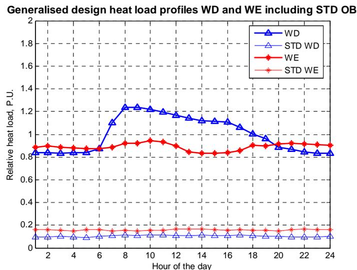
Figure 7.22 Generalised design heat load profiles for office buildings, weekdays and weekends, based on time control of the ventilation systems. The ventilation systems mainly run during working hours.
