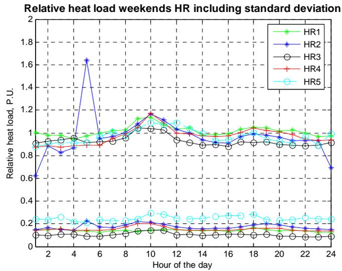
Figure 0.20 Design heat load profiles weekends for all HR analysed.
