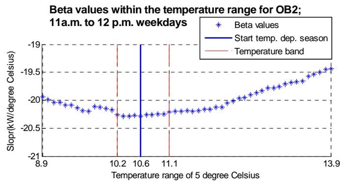
Figure 6.4 Beta values plotted within the  $5^\circ\text{C}$  temperature range found by the minimum total sum of squares of alpha values. The temperature band is given by the dotted lines and the start of the temperature-dependent season is given by the solid line.
