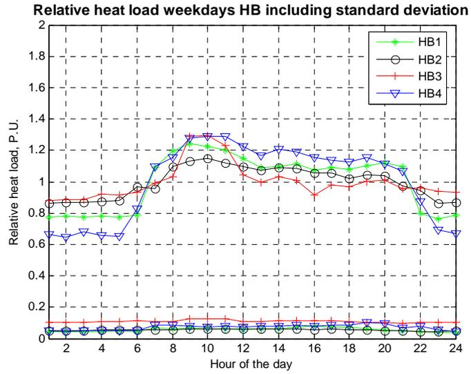
Figure 0.15 Design heat load profiles weekdays for all HB analysed.
