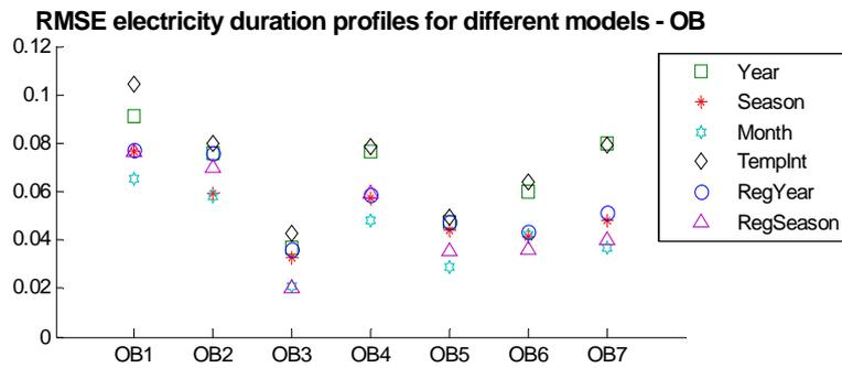
Figure 7.51 RMSE for calculated and real normalised electricity load duration profiles for all office buildings analysed.
