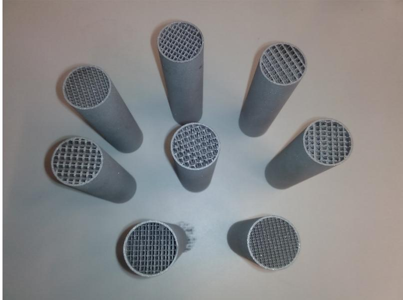
*Image 22: Samples of tubes with embedded lattice structures, 8 different designs*
