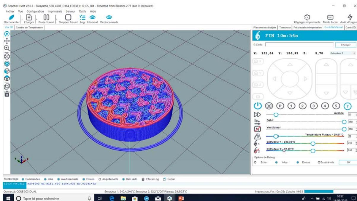
Image 10: Example of the Repetier display showing the 19 first layers of a 3D foam
