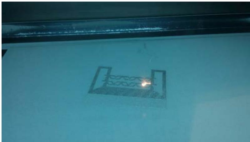
*Image 34: Printing process for the half section of the reactor*
