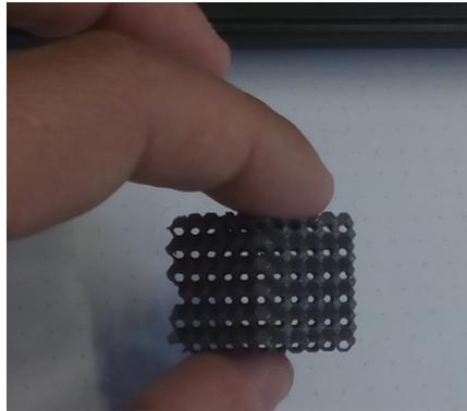
Image 21: Support less through holes in the Kelvin Cell structure
