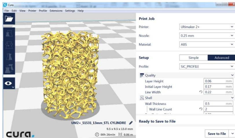
Image 5: Foam design in Cura software (Ultimaker 3D printer)
