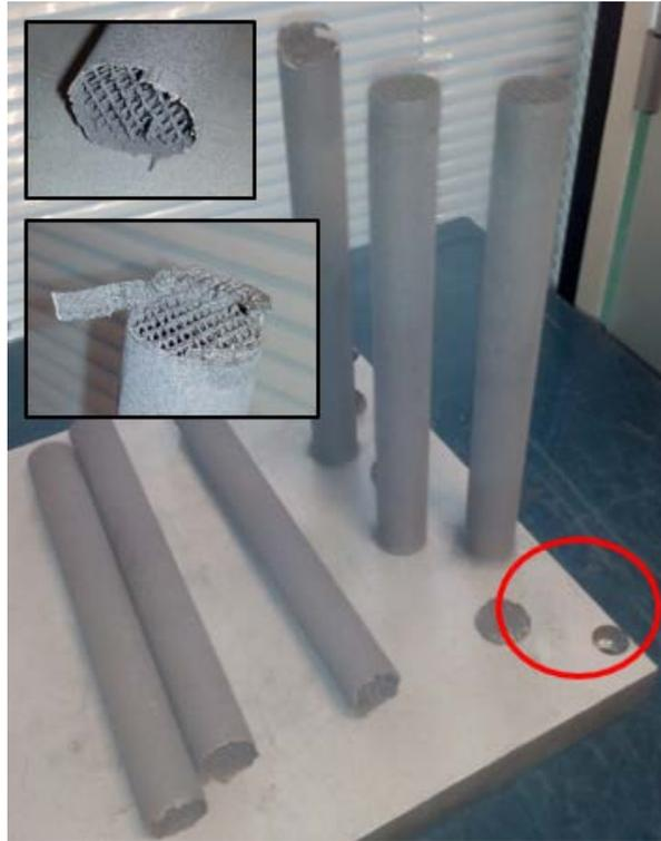
*Image 26: Breakage of the tubes from the building platform*
