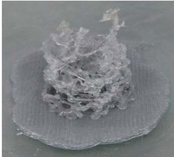
*Image 6: 3D printed foam obtained from tomography (ABS material)*
