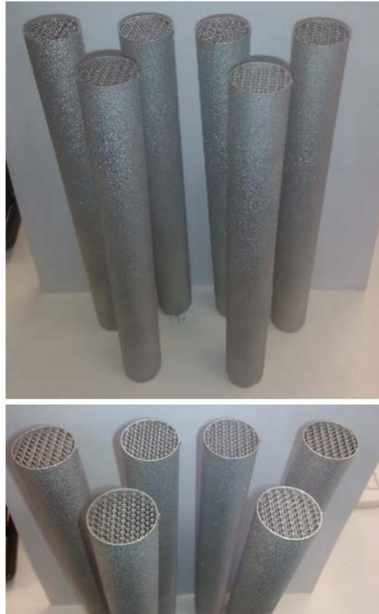
*Image 28: Batch of tubes printed after re design*
