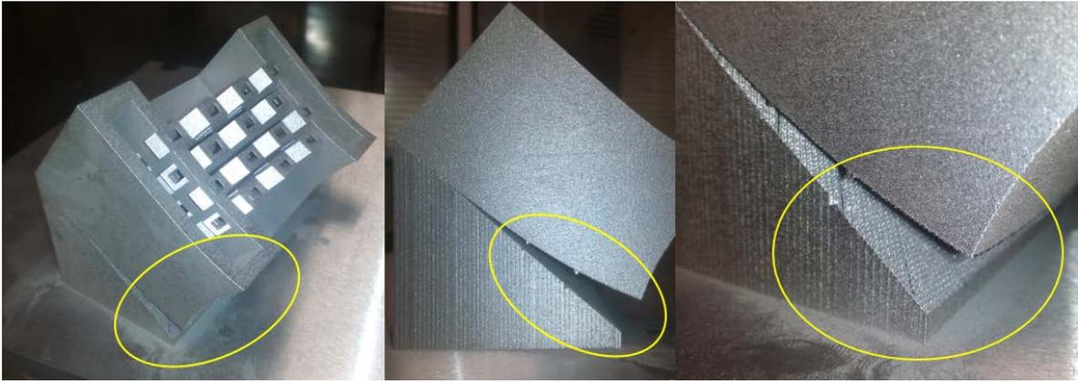
*Image 35: Printing results of first printing test*
