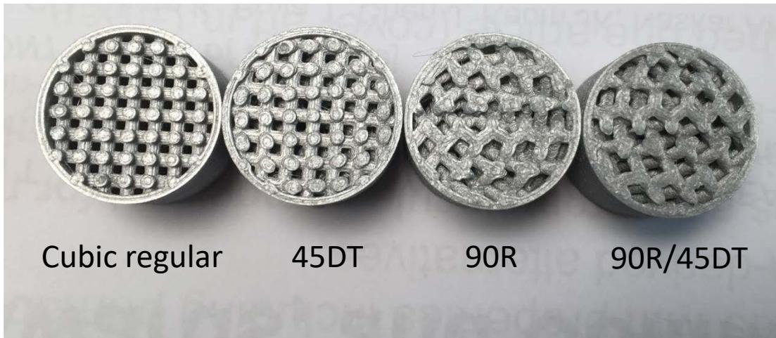
*Image 13: First 3D printed parts in ABS with 4 designs based on cubic cells*
