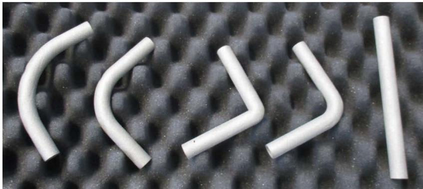
*Image 18: Final printed tubes, after supports removal*
