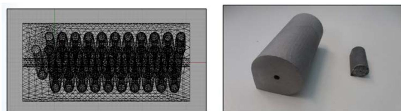
*Image 19: Internal design of the reactor (left) and comparison between original size and scaled model (both printed)*
