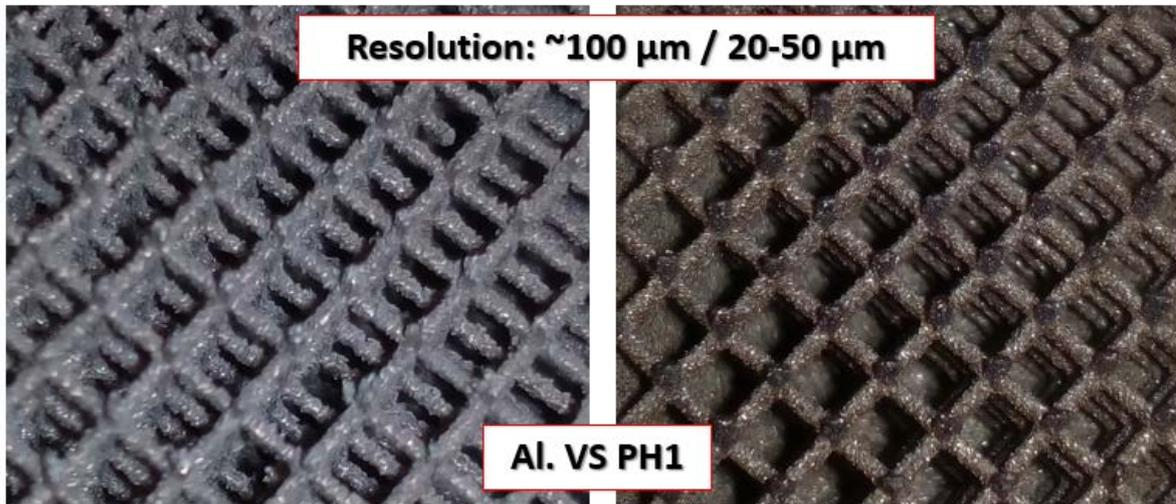
*Image 24: Aluminium mesh (left) vs Steel mesh (right). Differences in resolution and surface roughness can be seen*
