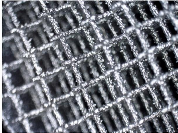
*Image 30: Mesh quality inside the lattice structure*
