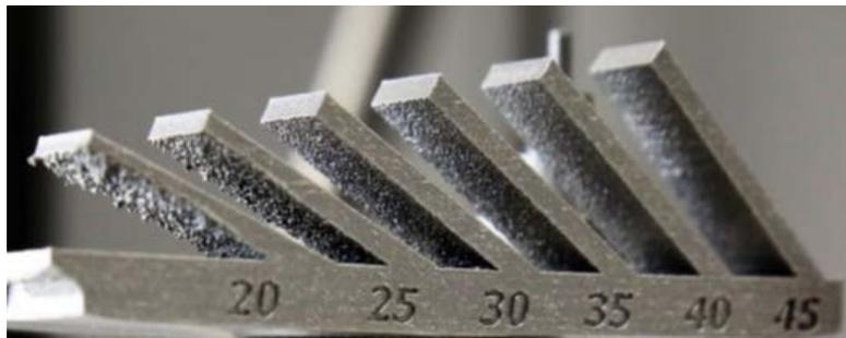
*Image 15: Dependence of angular design and material behaviour*
