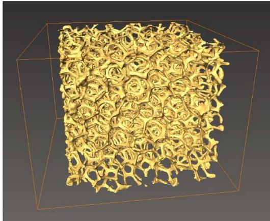
Image 3 : Reconstruction of the foam with ImageJ software
