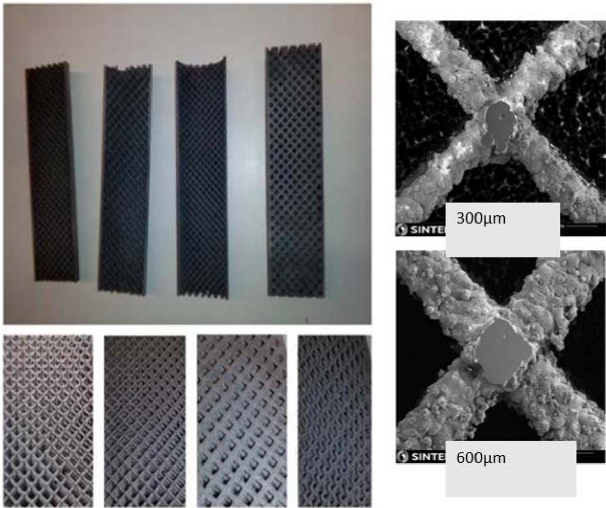
*Image 23: Half sections of the lattice tubes (left); microscopy pictures of the mesh walls (right)*
