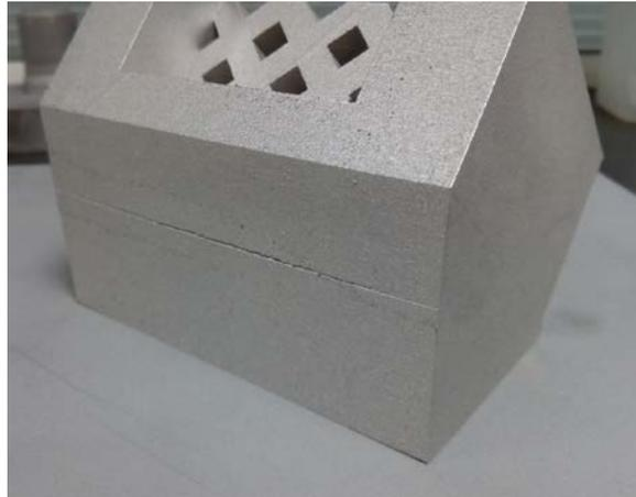
*Image 39: Defect in the third iteration of the printing cycle: internal cracks*
