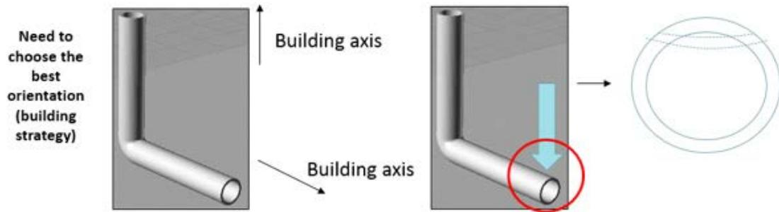
*Image 16: Selection of priority building axis (left): a main direction is going to be compromised. Effect of printing out of the building axis (right) resulting in geometric distortions*
