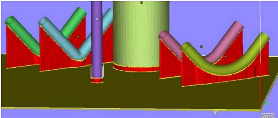
*Image 17: Nesting of burst pressure test specimens in Magics software*
