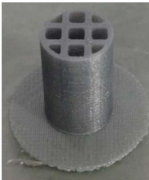
*Image 8 : 3D monolith used to establish printing design rules*
