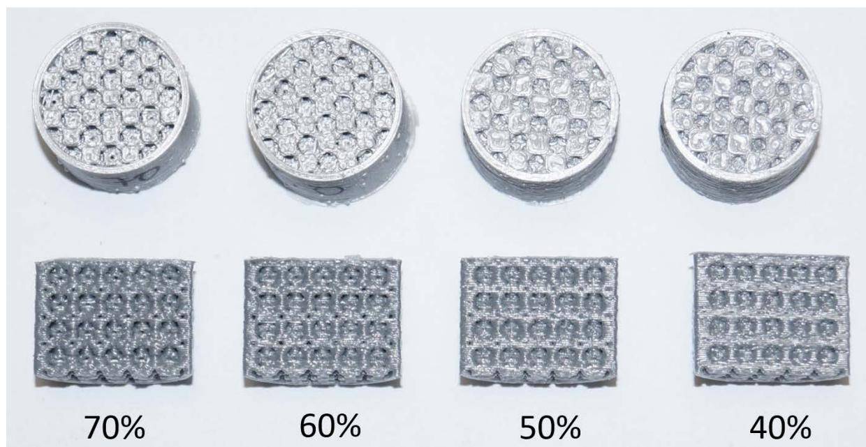
*Image 11: 3D printed parts in ABS with 4 porosities between 40% and 70%*
