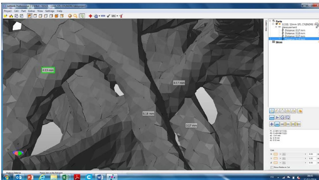
*Image 7 : Magnification of foam struts with Netfabb software*
