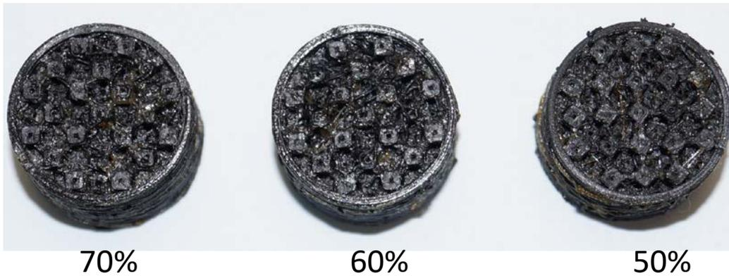
*Image 12: 3D printed parts with 3 higher porosities with PRINTCR3DIT formulated material*
