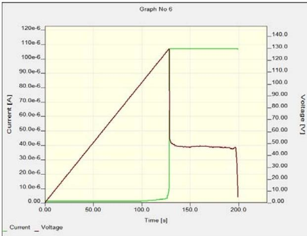
Figure 1.4: Breakdown test using voltage ramp of 1V/second, pad size
