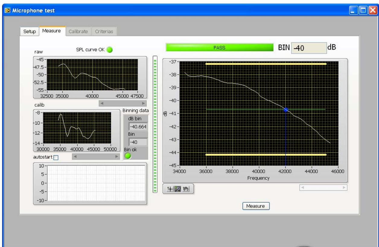
*Figure 19 Actual microphone sensitivity measurement on a ECM showing the result of compensating for the acoustic characteristics of the anechoic chamber.*
