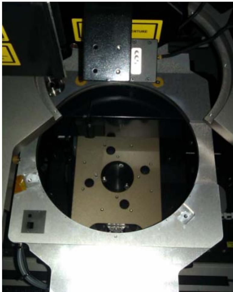
Wafer chuck of the aixDBLI tool with permanently mounted reference x-cut quartz. By mounting an insertion ring the system can be adapted to any wafer size
