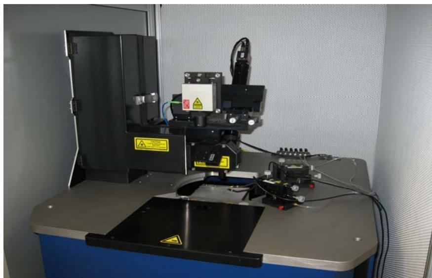
Figure 1.1.5: Inside view of the aixDBLI chamber without additional functionality of device testing and force measurement
