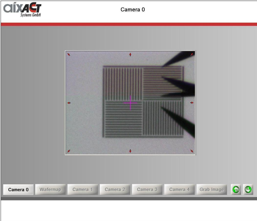
Figure 1.1.8: Wafer view camera picture of a alignment structure
