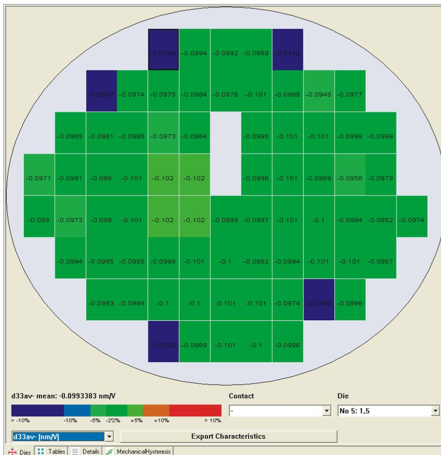
Figure 1.1.11: Wafer map view in the aixPlover software tool for statistical data evaluation
