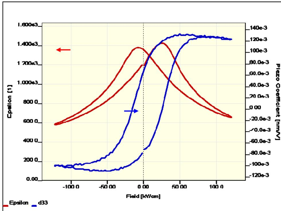
Figure 1.1.10: Test measurement of small signal dielectric and piezoelectric response vs. applied DC bias voltage of a PZT thin film sample
