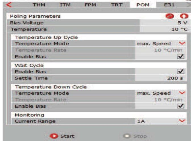
During the project the poling procedure has been identified as very important in view of the forming of the material in order to achieve very high piezoelectric coefficients. All the results that were derived during the project in view of different poling conditions were taken into account and realized within this software. Values up to  $e_{31,f}$  of almost 20 C/m<sup>2</sup> were achieved after poling. This is world record in published  $e_{31,f}$  values.
