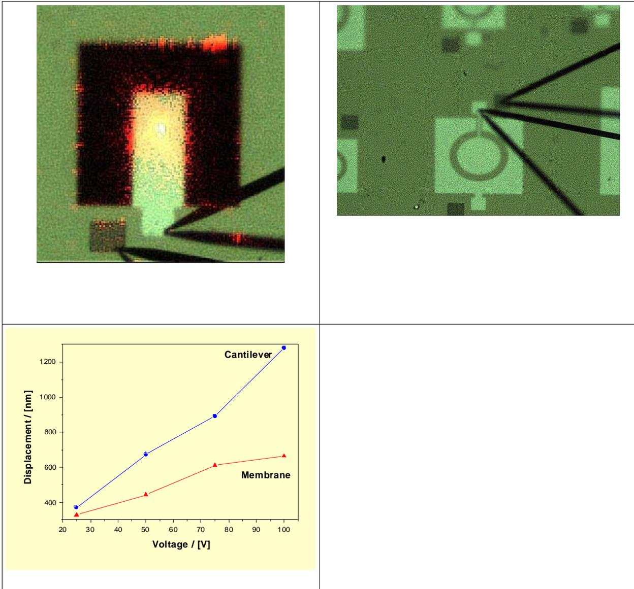
Cantilever and membrane structure to be tested by single beam functionality of aixDBLI system
