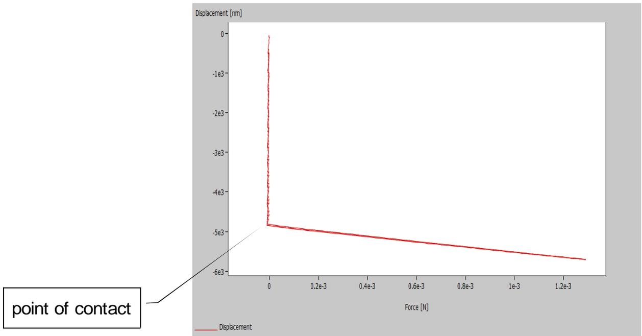
Blocking force measurement on a silicon reference sample utilizing the aixDBLI system
