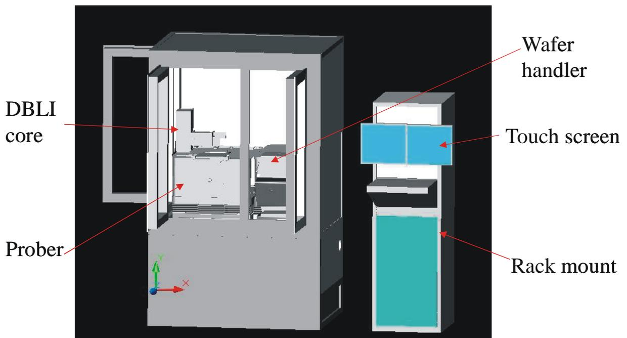
Figure 1.1.2: Schematic of the aixDBLI components
