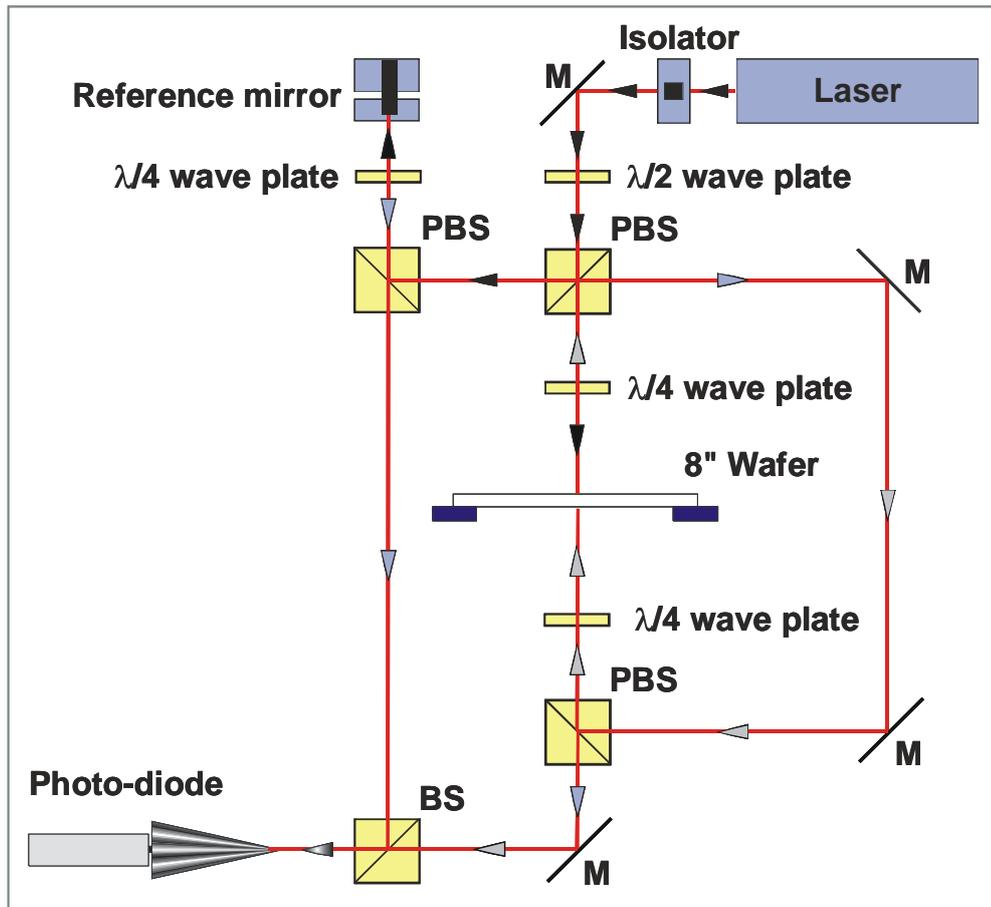
Figure 1.1.1: Double Beam Laser Interferometer optical path
