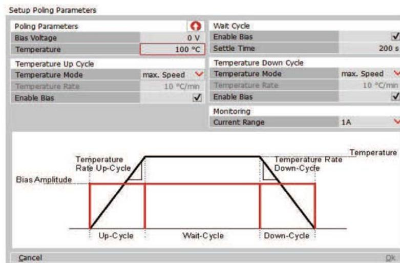
Advanced Poling Measurement dialog with parameter and excitation signal
