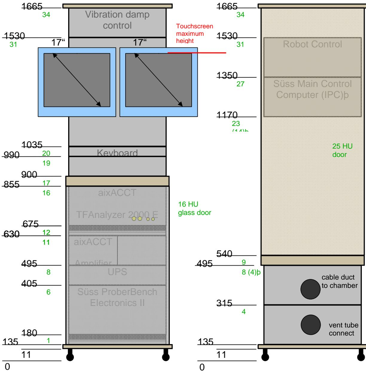
Figure 1.1.3: Components and dimensions of the rack mount (compliant with Semi standards S2 and S8)
