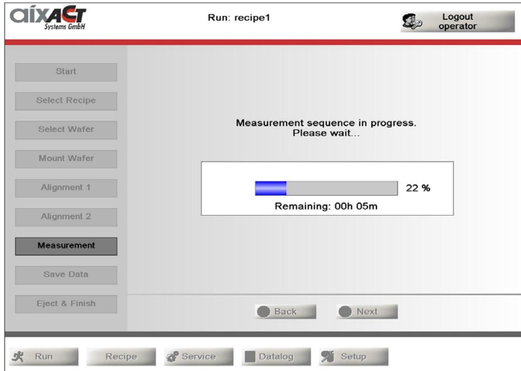
Figure 1.1.7: Graphical user interface of the measurement software operated by touch screen
