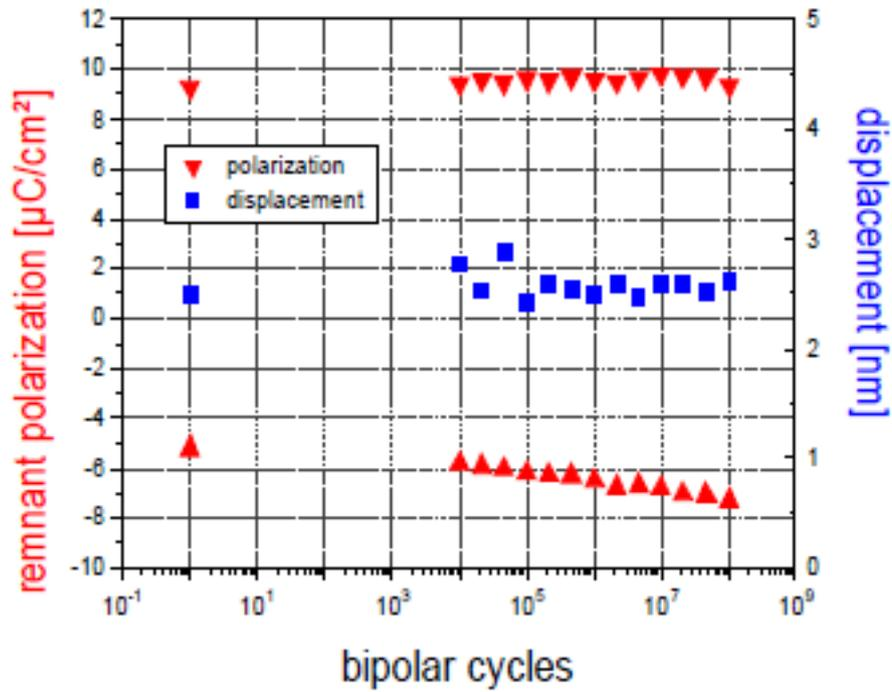
Fatigue data recorded utilizing treatment procedure
