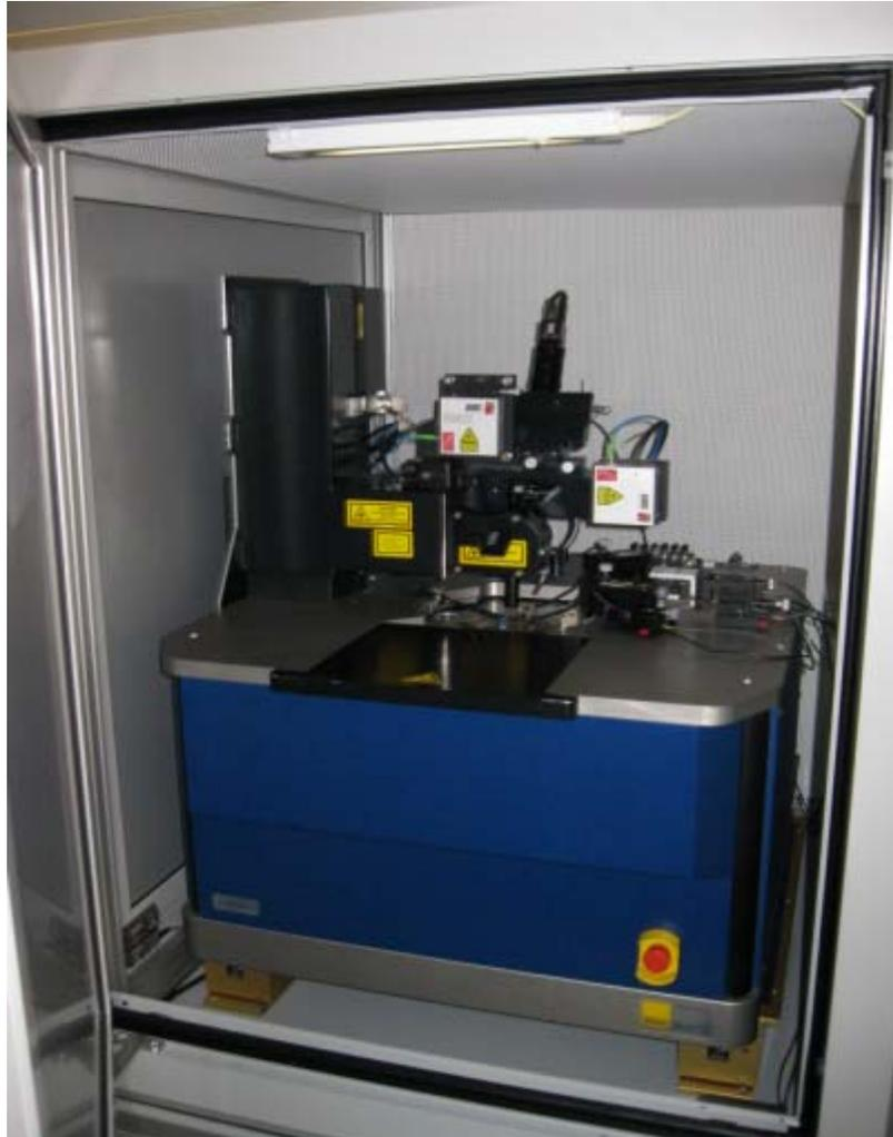
View inside the aixDBLI chamber, showing the chuck system and DBLI optics the single beam option and the force measurement unit.
