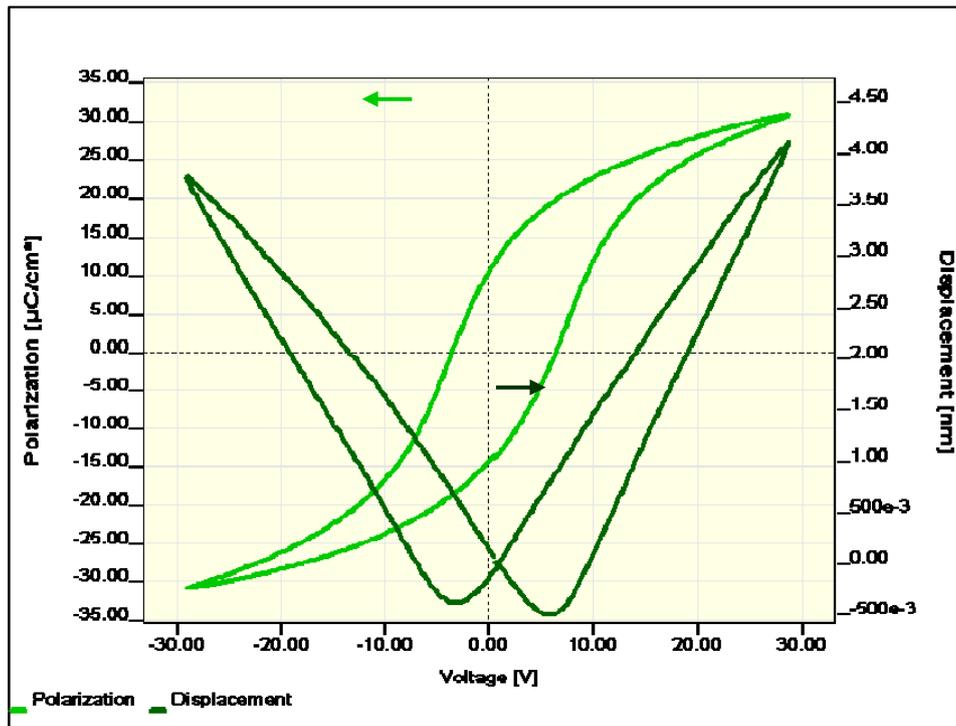
Figure 1.1.9: Test measurements of large signal polarization and displacement response vs. applied excitation voltage of a PZT thin film sample
