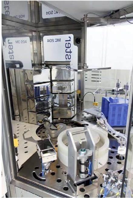
The picture to the left shows the inside of the CSD cabinet: coater, robot and hotplates (front to back). The original cover has been removed as it had been identified to be one cause for the particle problem experienced with the demo tool. Consequently the inner bowl was removed too, to lower the position of the wafer, which helps to avoid contamination of the cabinet by spun off fluid.
