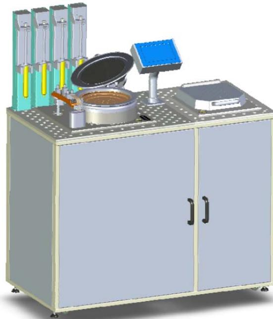
Fig. 1: Prototype CSD coater tool without RTP
