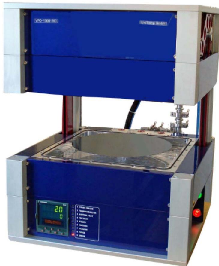
Fig. 2: Prototype of RTP furnace with cover opened and 300 mm wafer inside
