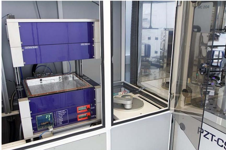
Fig. 8.: RTP, transfer robot and CSD coater (from left to right)
