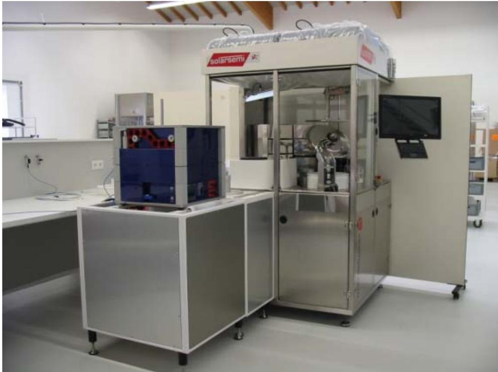
Fig. 3: Automated coating tool together with RTP-furnace during assembly at SOS
