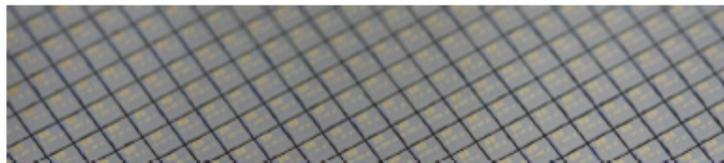
Figure 4.1: piezoVolume devices (also termed chips or dies) after the wafer has been diced.
