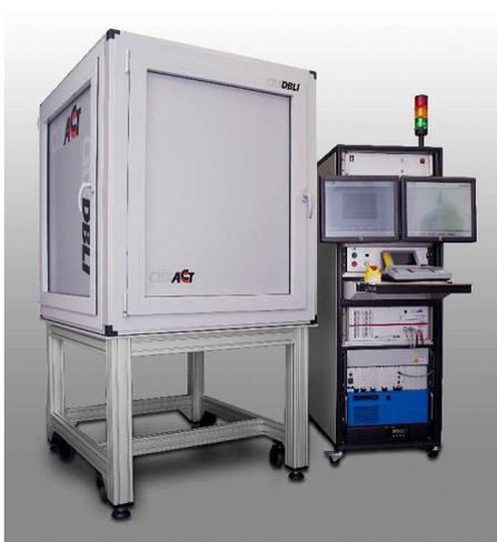
Figure 27: Picture of the assembled aixACCT aixDBLI system with isolation vibration chamber and electronic rack with operation control unit.
