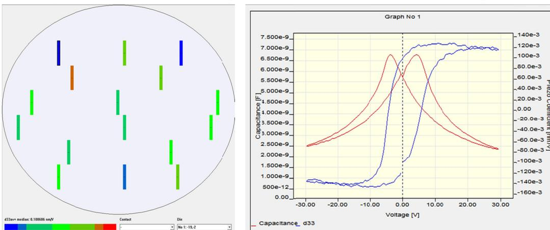
Figure 21: Uniformity of  $d_{33,av}^+$  and a combined C(V) and  $d_{33,f}$  measurement for one pad
