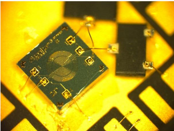
Figure 39: Microphone mounted with FETs for measurements
