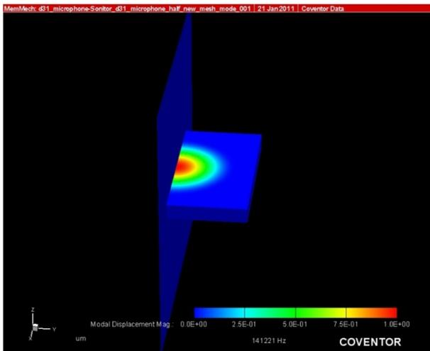
Figure 37: Coventor simulation results of the 3D eigenmode analysis with the frequency and shape of the first eigenmode.
