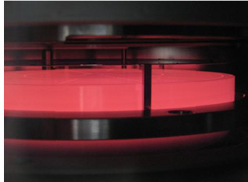
A maximum temperature of more than 800°C is achievable with the very hot chuck which is well above the chuck temperature range of 550 - 700°C necessary for in-situ deposition of PZT. Therefore the very hot chuck can also be utilized to deposit other materials which need an even higher temperature to grow in-situ in the required crystal structure such as BaSrTiO<sub>3</sub> (BST).
