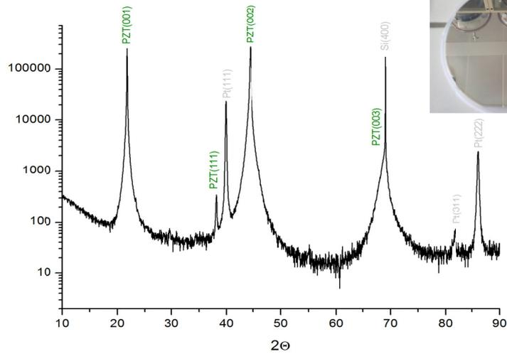
Figure 10: Crystallographic analysis of a 2  $\mu\text{m}$  thick PZT film
