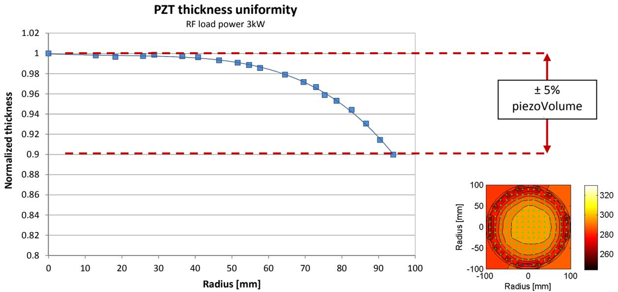
Figure 26: Thickness uniformity of PZT film deposited at 3 kW
