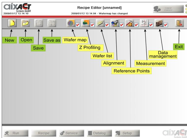
Figure 29: Screen shot of the Graphical User Interface of the aixDBLI system on touch screen basis.
