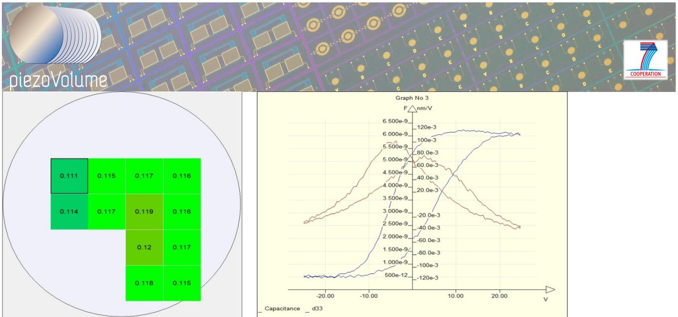
Figure 7: Wafer map of pV066 with distribution of  $d_{33,max}$  over the wafer prepared by the low temperature route. The measured  $d_{33,max}$  values are high and very homogeneous over the wafer.
