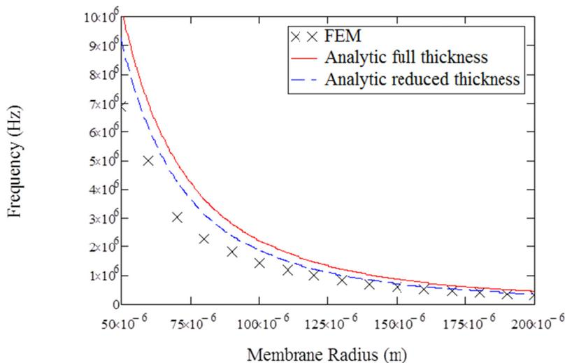
Figure 36: Resonance frequency as function of membrane radius. The red curve shows the analytical results based on the mass and flexural rigidity of the full stack, whereas the blue broken curve is based on the mass and flexural rigidity of the (Si-SiO<sub>2</sub>-Pt only).
