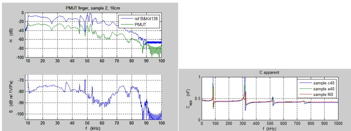
Figure 40: piezoMEMS microphone sensitivity measurements and frequency sweep showing resonance frequencies.
