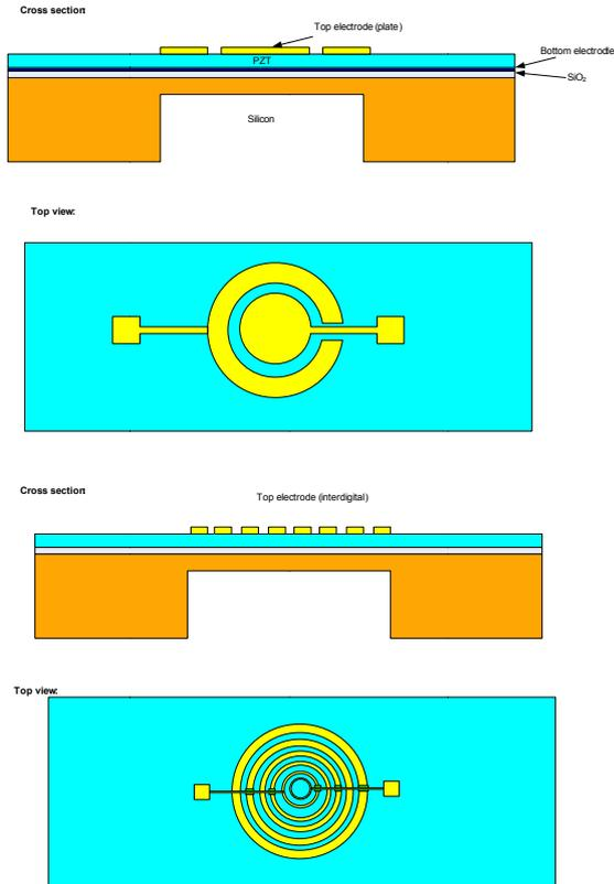
Figure 35: Cross-section of the two  $d_{31}$  and  $d_{33}$  variants for microphones/actuators, with and without bottom electrode.
