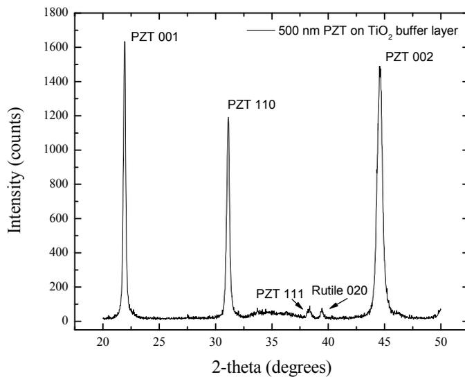
Figure 8: X-ray diffractogram of a 500 nm PZT thin film prepared deposited on the  $TiO_2$  buffer layer.
