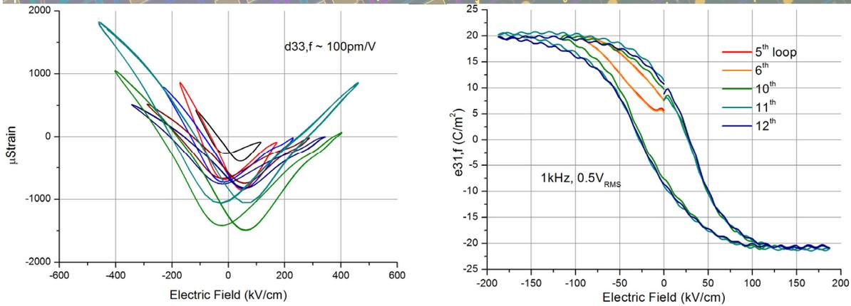
Figure 12: Determination of piezoelectric constant  $d_{33,f}$  by Stain vs.  $E$ -field measurements under large signal excitation (left), Small signal  $e_{31,f}$  vs.  $E$ -field measurements (right) for a  $2 \mu\text{m}$  thick PZT film
