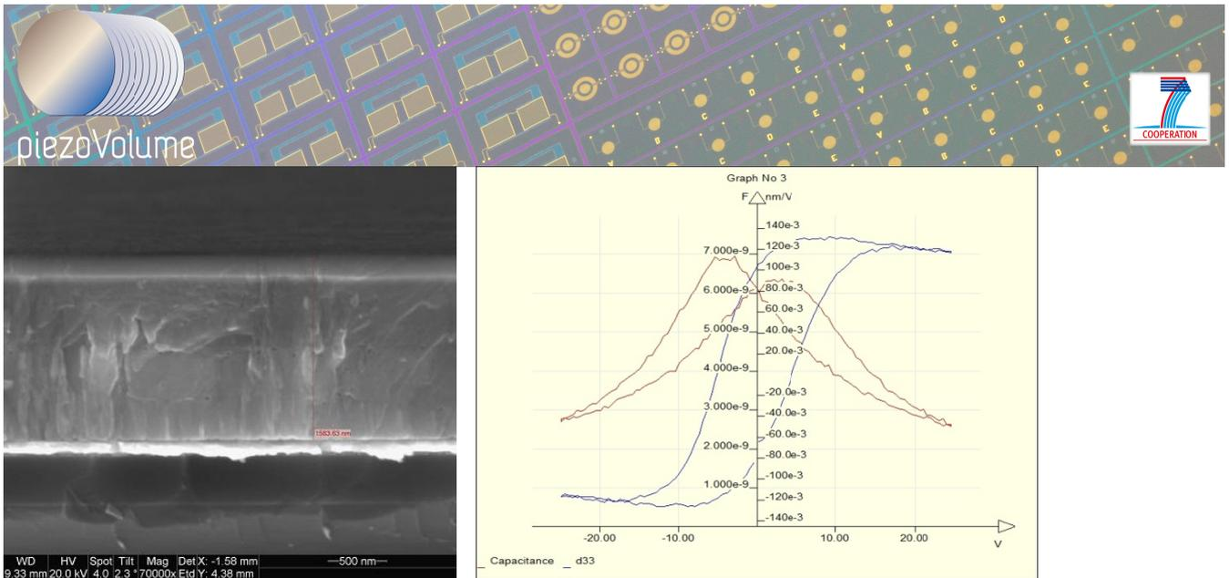
Figure 5: A 2 $\mu\text{m}$  PZT film deposited using a modified formulation and resulting high  $d_{33,f}$  performance
