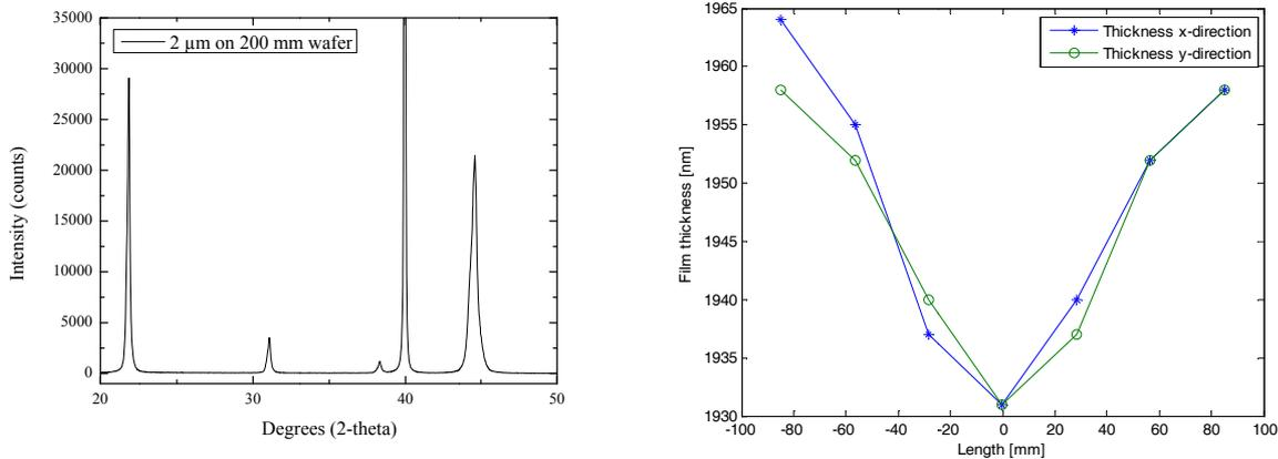
Figure 20: X-ray diffractogram of the center area of the 200 mm wafer and thickness uniformity measured by ellipsometry
