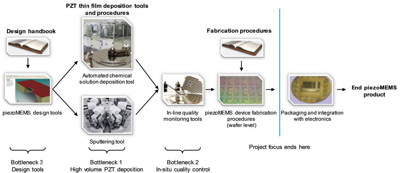
Figure 1: The piezoVolume process chain
