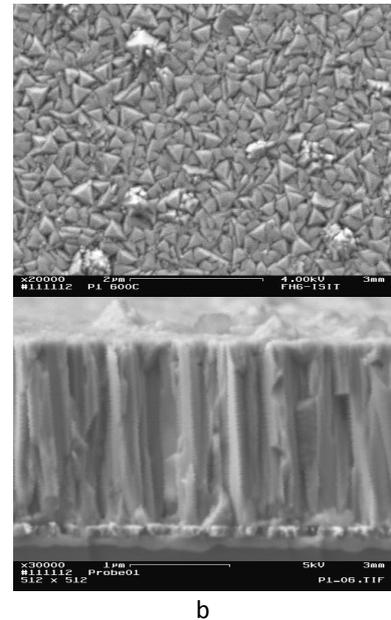
Figure 13: a) XRD analysis of a  $2 \mu\text{m}$  thick PZT film deposited on a 200 mm substrate, inset: patterned wafer used for ferroelectric, piezoelectric and dielectric characterization; b) surface and cross section of a PZT film
