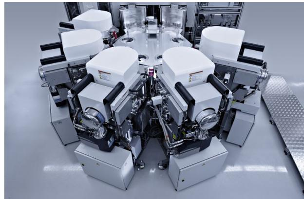
The sputter module to deposit PZT by RF magnetron sputtering on 150 mm or 200 mm wafer consists of a vacuum chamber equipped with a turbo pump, a RF sputter cathode with impedance matching network and a impedance matching network for application of RF bias to the substrate (Figure 23).
