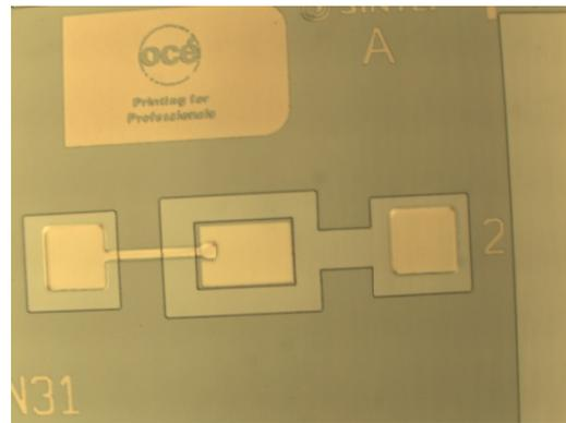
Out-of-plane deflection was measured using Polytec SLV with MSA-400 optical measurement head. Additionally this setup was used for evaluation of the device stability/reliability.
