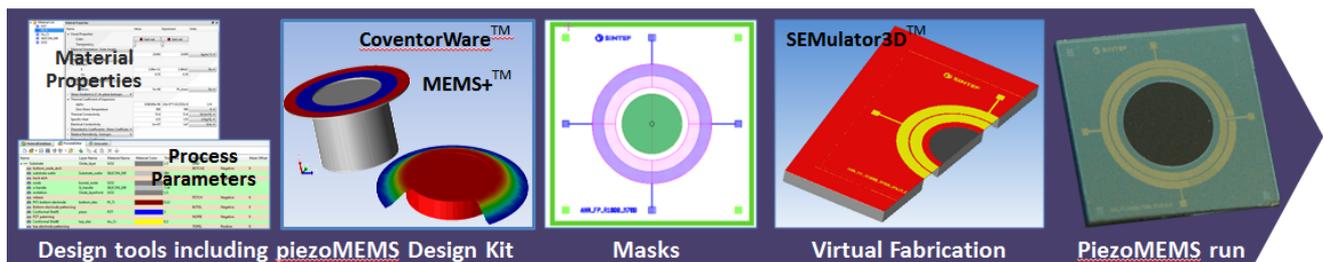
Figure 32: Design flow and modelling levels included in the PDK for MoveMEMS PZT.
