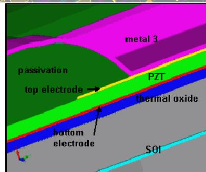
Figure 34: Ultrasonic transducer from Vernon generated by SEMulator3D with its comparison to a photograph and a cross section
