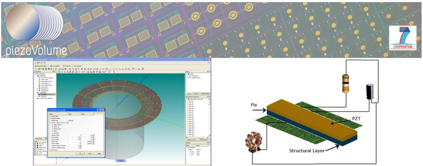
Figure 31: New shell model (left) and Schematic representation of a FEM cantilever including connection of simple circuit elements (via boundary conditions).
