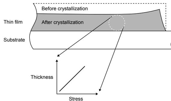
Figure 4: non-uniform shrinkage during drying of thin film layer
