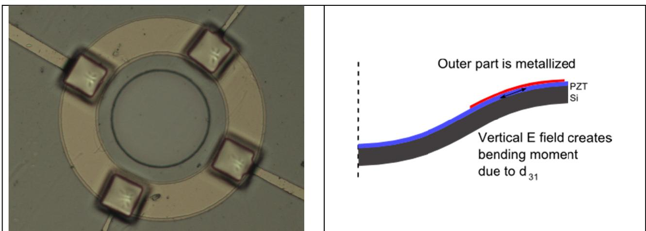
Figure 41: View of a Vernon pMUT device (left), and snapshot of the working principle of a pMUT membrane (below).
