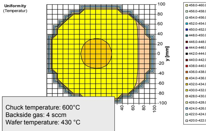
Figure 25: Temperature distribution on a sense array test wafer at heater set point 600°C.
