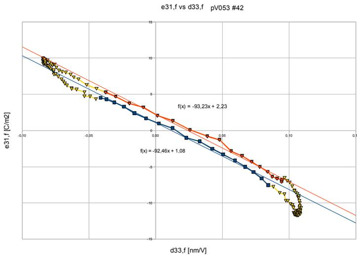
Figure 30: Correlation of  $e_{31,f}$  and  $d_{33,f}$  with slope of  $c_{13}$  enables indirect control of  $e_{31,f}$  by monitoring  $d_{33,f}$  and  $\epsilon_{33}$
