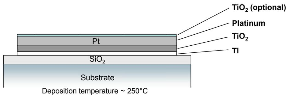
Figure 2: Bottom electrode layer stack
