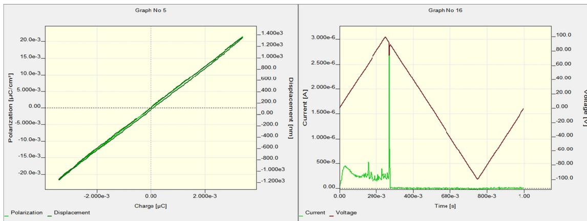
Figure 6:  $e_{31,f}$ : -15 C/m<sup>2</sup> at zero bias using modified coating formulation. Breakdown test at 1 Hz for small pad. Breakdown observed at 460 kV/cm.
