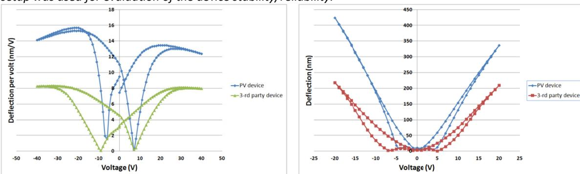
Figure above shows the small signal deflection (left), and large signal deflection (right). Blue lines represent the deflection measured on PiezoVolume devices while the red one corresponds to the deflection of the identical device but with the PZT layer from the third party. Clearly, PZT material developed with PiezoVolume project is twice more efficient than the material used in the previous experiments at Océ.
