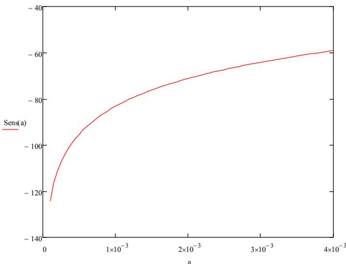
Figure 38: Sensitivity in dB (0dB is 1V/Pa) as a function of the membrane radius.
