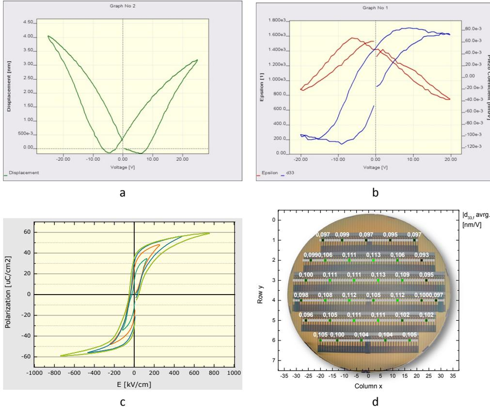
Figure 14: Piezoelectric response of PZT films of 2  $\mu\text{m}$  thickness for large signal (a), small signal (b) excitation; c) measurements of ferroelectric hysteresis loops; d)  $d_{33,f}$  mapping on a 200 mm substrate
