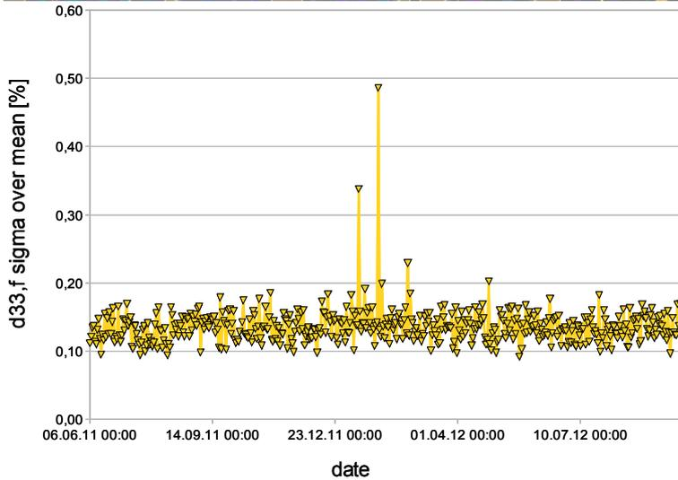
Figure 28: Sigma over mean data over 17 month of the aixDBLI system, which provides unique resolution and long term stability.
