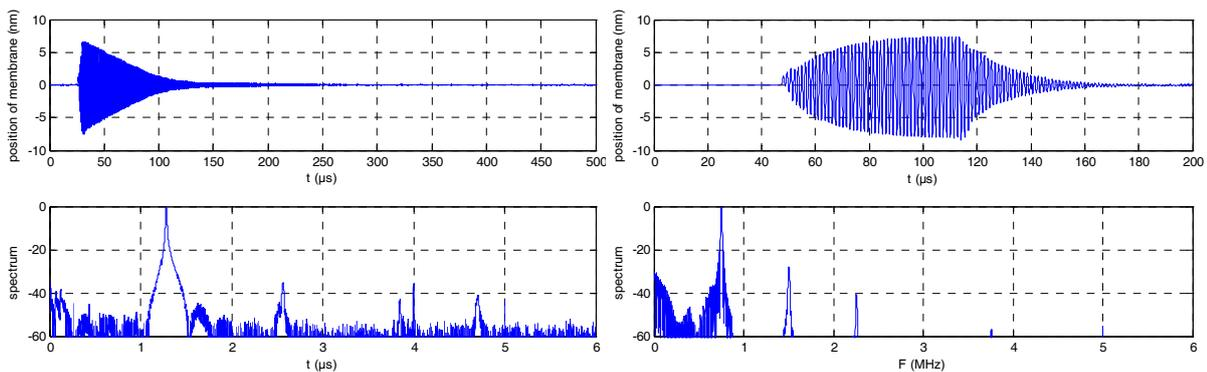
Figure 43: Results in air for a single 2.5 MHz pulse of 10 Vpp (left) 750 kHz, 20 Vpp, 50 cycles excitation in oil (right)
