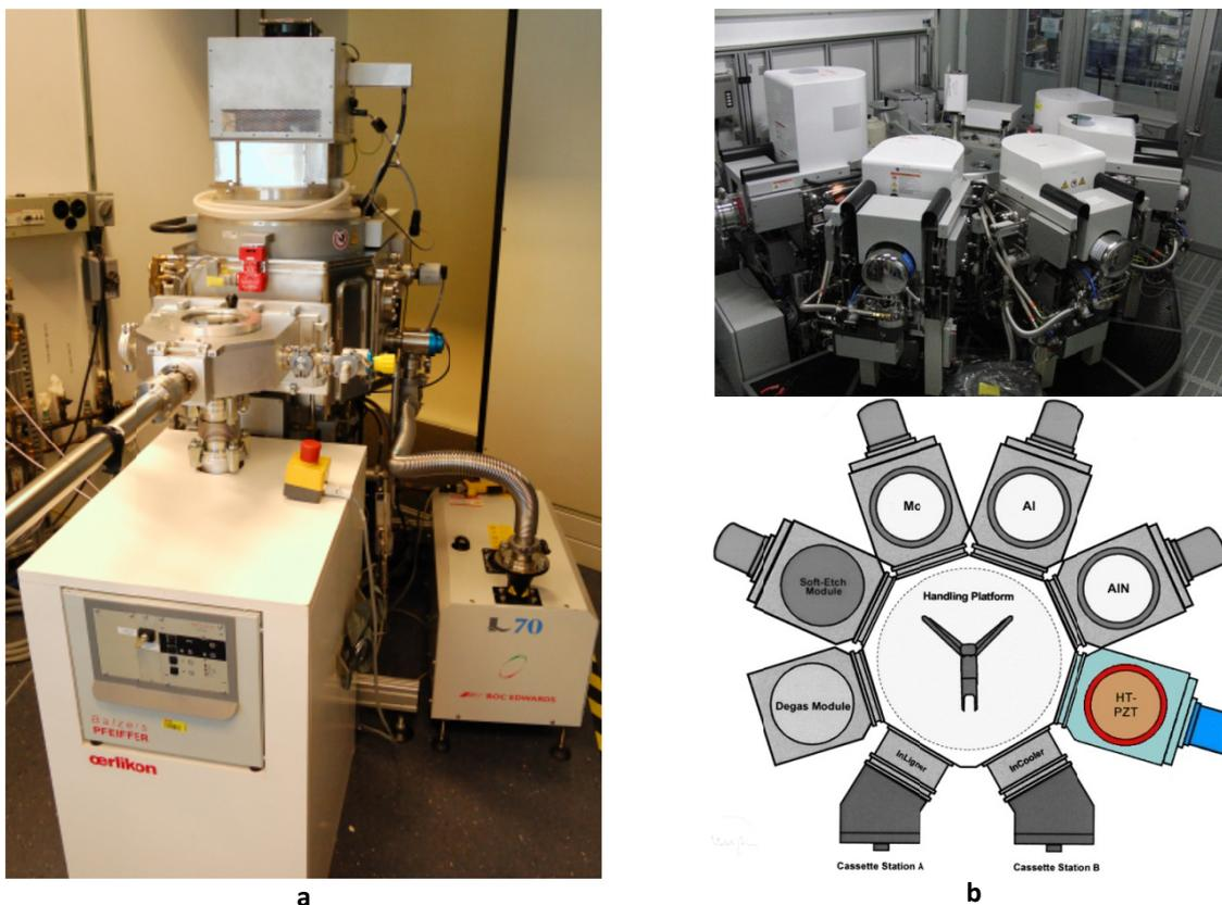
Figure 9: The two set up PZT sputter deposition tools; a) 150 mm PZT module located at EPL; b) 200 mm PZT module integrated in a CLN200 cluster tool located at Fraunhofer ISI
