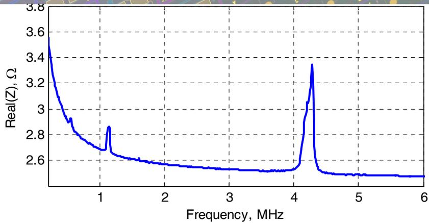
Figure 42: Impedance response (real part) of an element, displaying two resonance mode. The one used for ultrasonic transduction is around 1 MHz.
