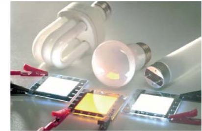
Fig. 3.4.15 OLED light sources have the potential to replace today's conventional light sources © Philips
