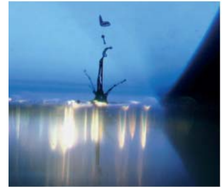
Fig. 3.3.7 Example for dynamic handling of cells, using laser pressure catapulting technology to take out a specific cell out of the tissue with no biological contamination © PALM
