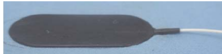
Rubber electrode, Mühlsteffa and Such, IEEE EMBS 2004
