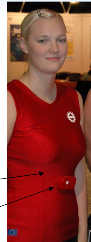
Textile electrodes sewn inside the fabric
