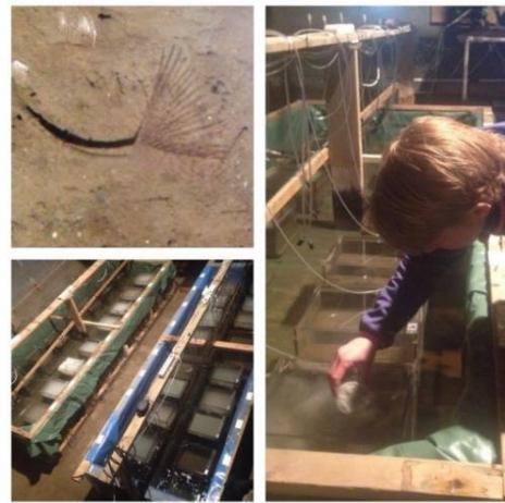
Figure 9. Deployment of the box core (left) to collect benthic communities for experimental studies (right) in NIVA's Solbergstrand mesocosm facility.
