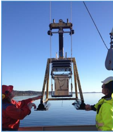
Figure 9. Deployment of the box core (left) to collect benthic communities for experimental studies (right) in NIVA's Solbergstrand mesocosm facility.
