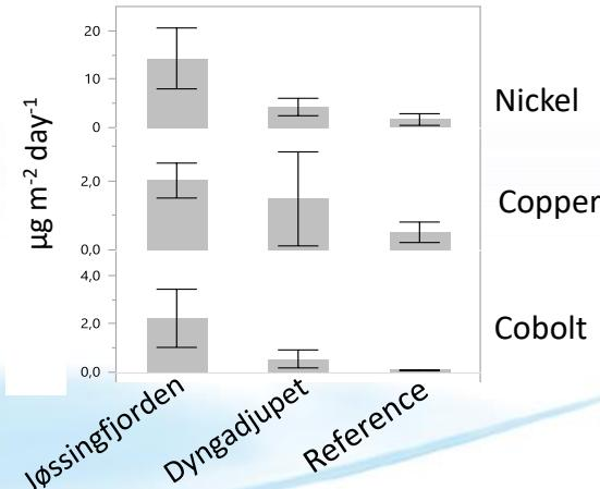
Flux of nickel from sea deposits corresponded to 5.2% of leakage from land deposit
