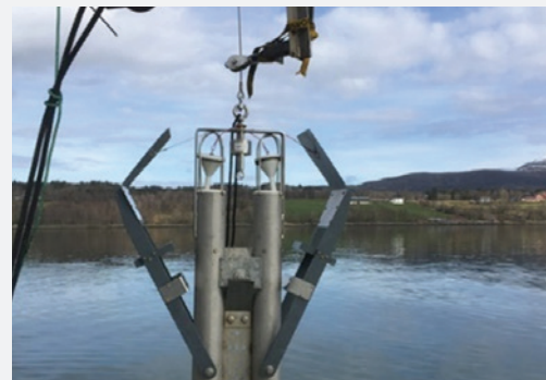
Sediment samples from Frænfjorden (left) where taken using a Gemini corer (right). Photo: E. Ramirez-Llodra (NIVA).
