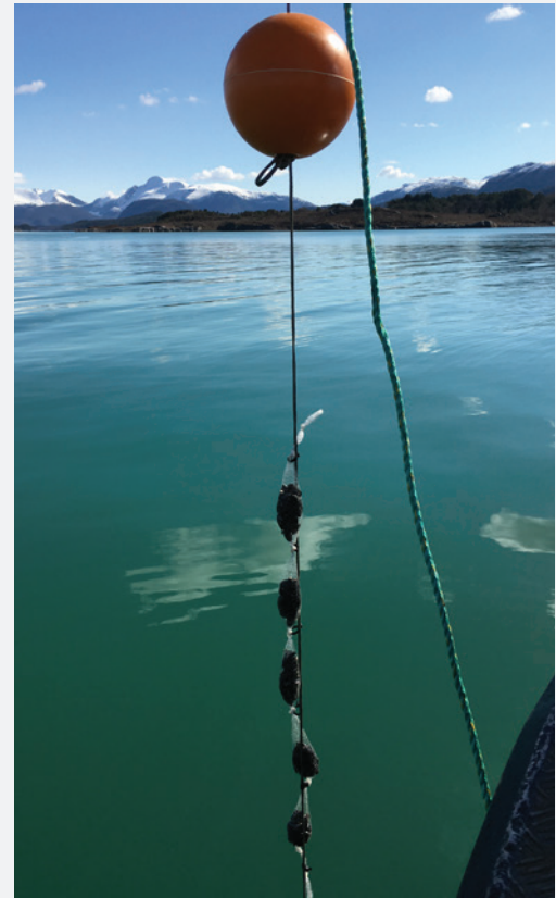
Deployment of mussels in a fjord recipient to study environmentally relevant impacts of the tailings to mussel health and chemical bioaccumulation.
