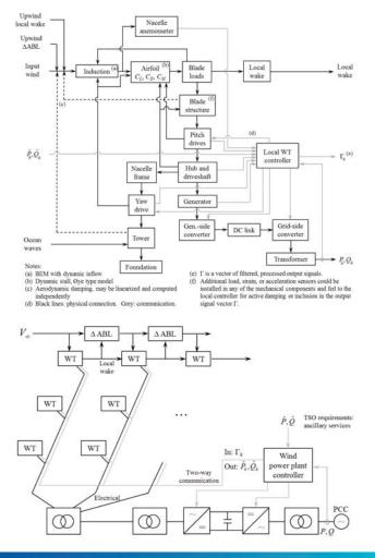
Accurate prediction of electrical/mechanical/control interactions (subsynchronous resonance) requires a complete model of the plant, with good models of both the mechanical and electrical systems.
