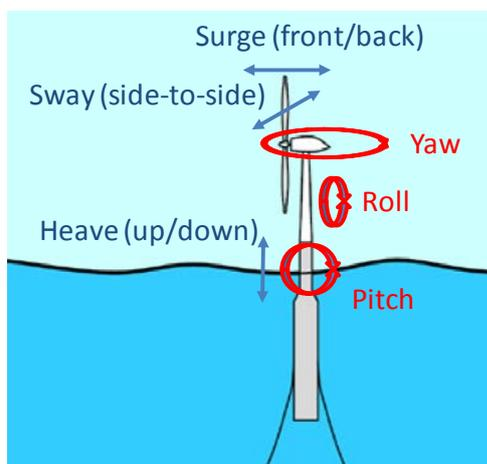
The motions of a floating wind turbine are defined by the six degrees of freedom:
