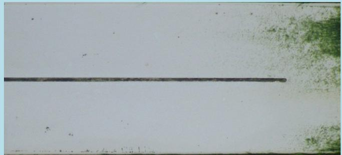
Coating systems combining thermal sprayed zinc and a paint applied in 1-coat instead of a conventional 3-coat paint system show promising corrosion performance in a field test at Helgoland.
