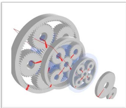
**Illustration of torsional model of a 5 MW wind turbine gearbox for internal dynamic investigation of gears.**
