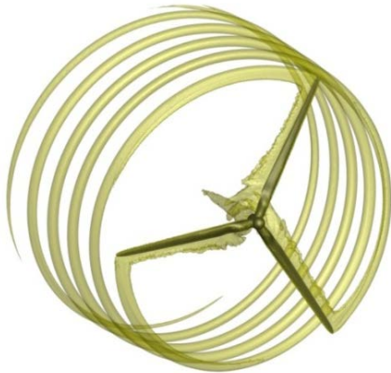
Vorticity field simulated with the TAU-DLR code behind the NREL 5MW reference turbine
