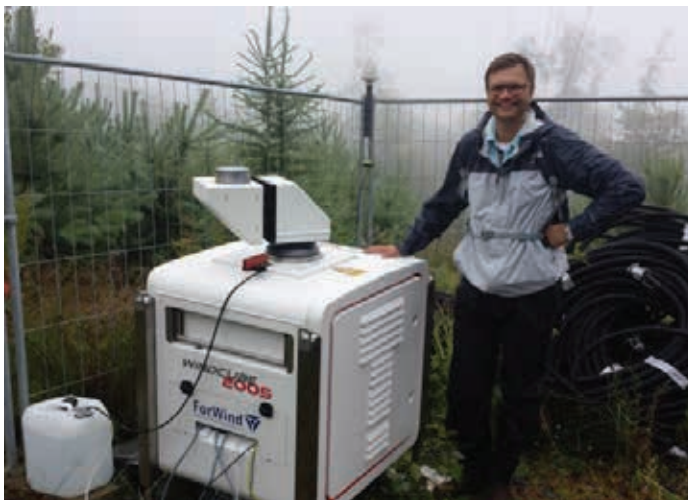
Figure 31: A system test with 6 Lidar Wind Scanners were made in Kassel in Germany in the summer of 2014. The lidar units were placed around Rödeser Berg close to Kassel where a 200 m wind measurement mast offered an ideal test site for the Wind-Scanner facilities in complex terrain. The purpose was to prove the concept of several synchronized wind-scanning LiDARs as virtual meteorological masts in complex terrain.
