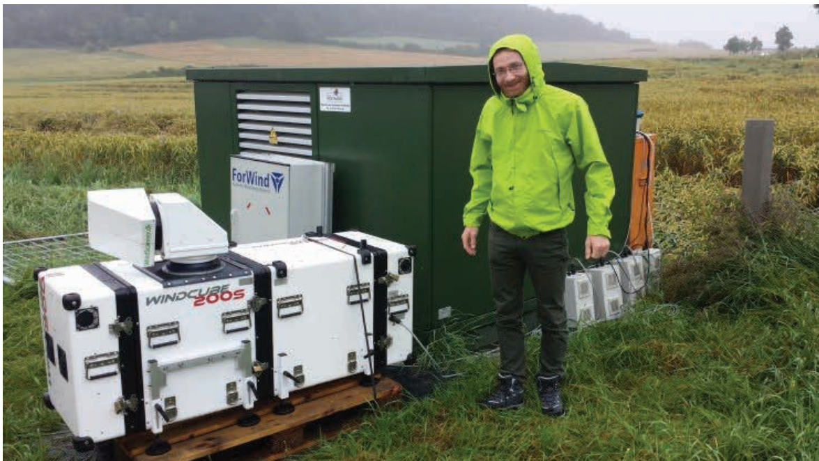
Figure 31: A system test with 6 Lidar Wind Scanners were made in Kassel in Germany in the summer of 2014. The lidar units were placed around Rödeser Berg close to Kassel where a 200 m wind measurement mast offered an ideal test site for the Wind-Scanner facilities in complex terrain. The purpose was to prove the concept of several synchronized wind-scanning LiDARs as virtual meteorological masts in complex terrain.
