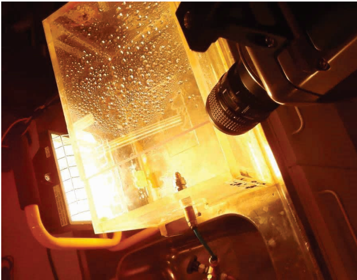
Figure 25: Laboratory setup for droplet erosion testing of blade coatings.
