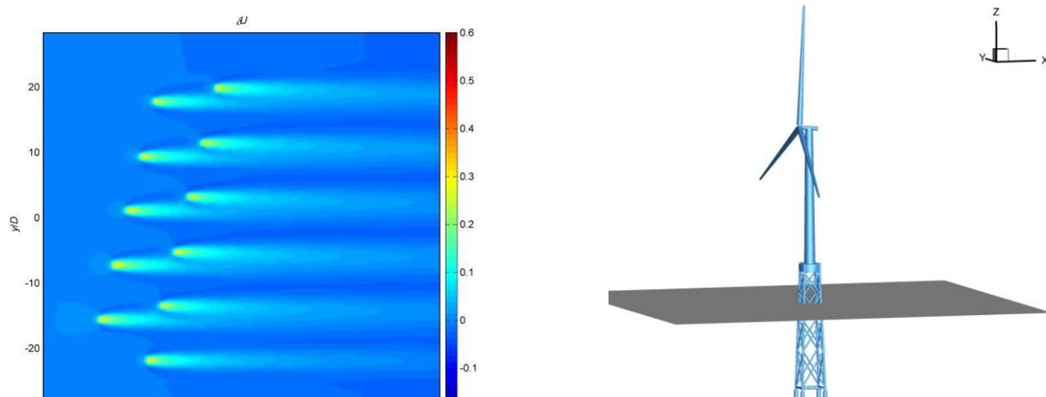
**Figure 8** 3D CFD wake simulation of Vindeby offshore wind farm compared well with measurements (left). Integrated simulations of jacket offshore wind turbines with NOWITECH developed software performed well in the international comparison IEA Annex 30 OC4 (right).
