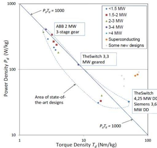
**Figure 10** Map showing power density vs. torque density for electrical generators for offshore wind turbines.
