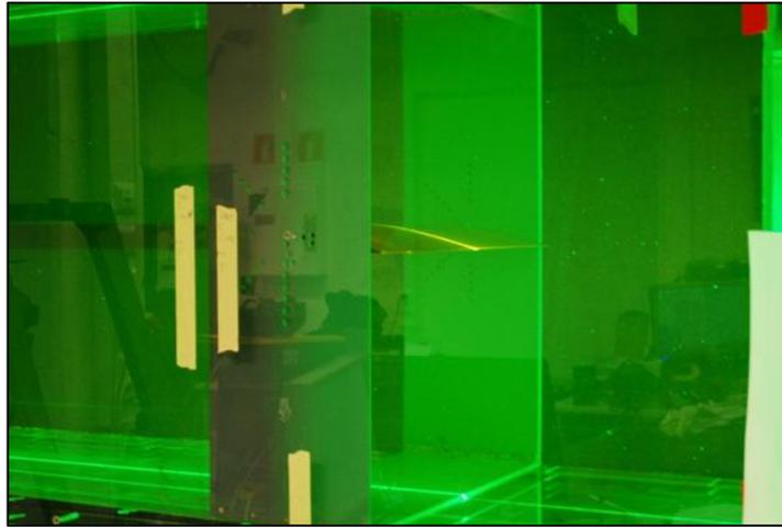
**Figure 15** An airfoil model mounted wall-to-wall in the circulating water tank for PIV-experiments. The experiment was carried out to investigate the effect of scaling in model tests. The measurement plane is vertically orientated in mid-span position.
