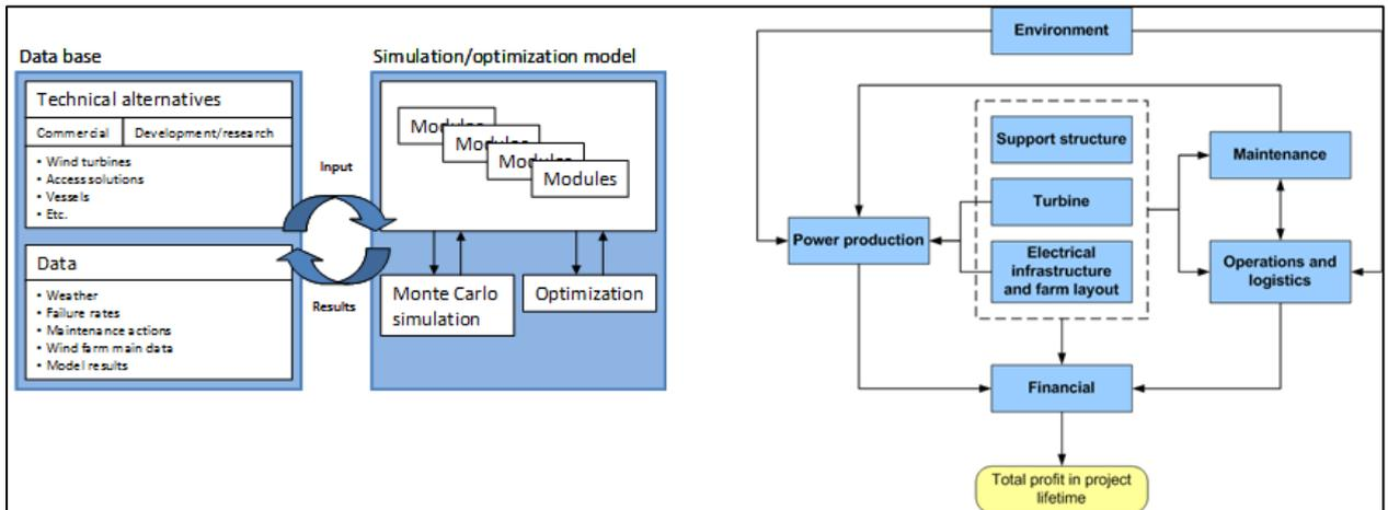
**Figure 13** Holistic/integrated model concept for Life Cycle Profit analysis of an offshore wind farm, including all phases from design to decommissioning (Task 5.1).
