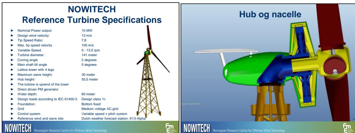
**Figure 7** NOWITECH reference turbine. Summary of specifications (left) and extract from hub and nacelle construction (right).
