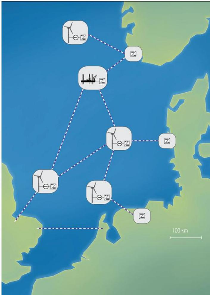
A North Sea multi-terminal high voltage DC grid has the potential to improve security of supply when interconnecting offshore wind farms and oil and gas platforms with the European power grids:
