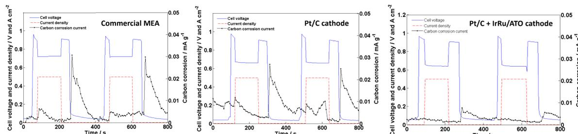
The AST consists in current cycling between 0 and 0.5 A cm<sup>-2</sup>, at 70 °C and using fully humidified gases. For each cycle the fuel cell is shut-down by purging the anode side of the fuel cell with air in order to removed t remaining hydrogen. FTIR measurements show that the hydrogen/air front at the anode induces carbon corrosion at the cathode. FTIR also shows that evolved CO<sub>2</sub> is considerably lower in magnitude for the IrRu containing electrode.
