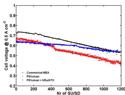
The IrRu containing Pt/C cathode shows considerably lower degradation rates, e. g. lower degradation of the ECSA and an overall lower voltage decrease, compared to the Pt/C electrode. For comparison, the same was performed with a state-of-the-art commercial MEA.
