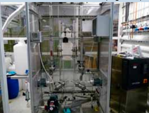
Figure 4: 10kW / 50barg test rig for PEM electrolysis stack at Fraunhofer ISE
