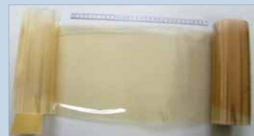
Figure 2: 5.5 sqm sPEEK membrane cast from UoR onomer
