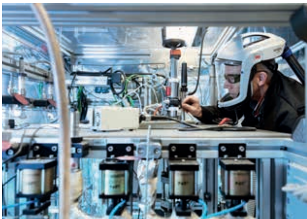
Measurements of phase equilibria using the ECCSEL CO 2 Mix facility of SINTEF Energy Research
