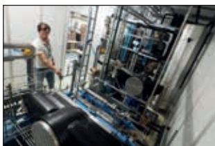
The ECCSEL well integrity research infrastructure. This mini-wellbore simulator is used for in-situ investigation of cement integrity under CT imaging. Sketch by A. Ghaderi.
