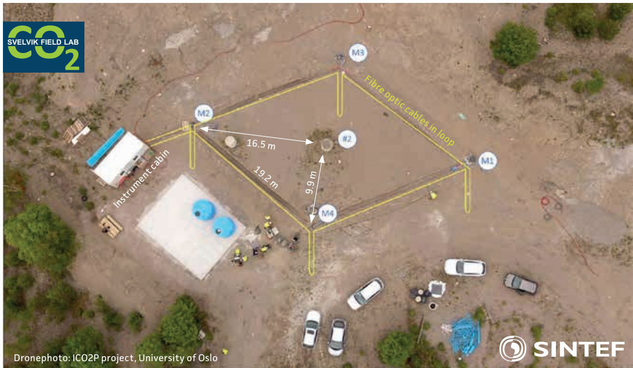
Aerial view of the Svelvik CO 2 Field Lab with injection (#2) and monitoring wells (M1-M4) marked. The loops with fibre optic cables (several different commercial and research types) are shown yellow with "tongues" indicating how the cables also go down into the wells.
