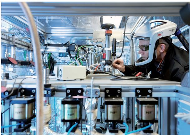
*Measurements of phase equilibria using the ECCSEL CO<sub>2</sub>Mix facility of SINTEF Energy Research*
