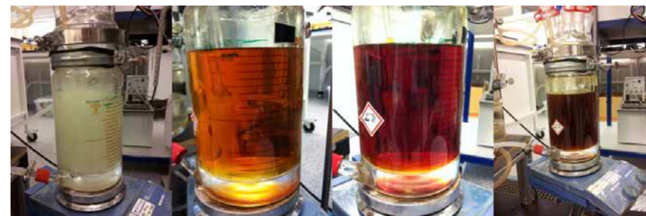
Initial 20 hrs 93 hrs 187 hrs Example on solvents colour change for an oxidative degradation experiment.
