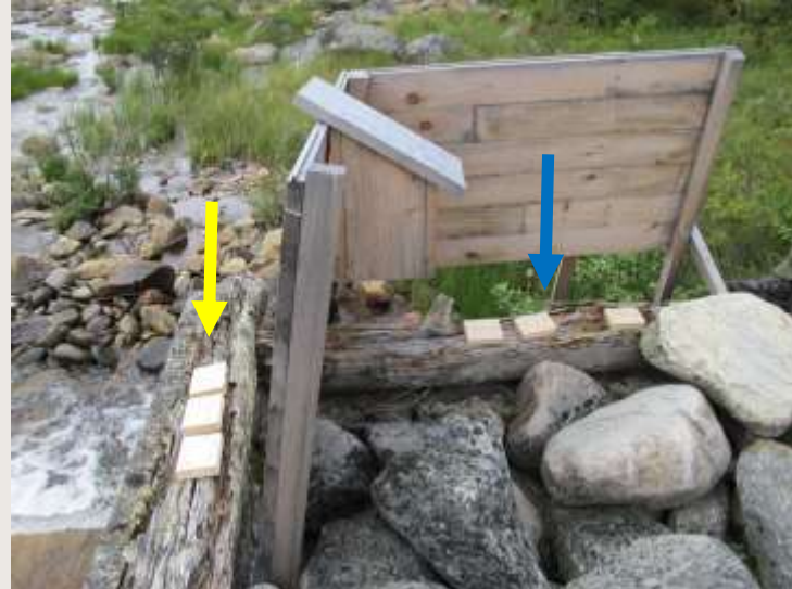
Fig. 114. Detail of Fig. 113. Test of variation of temperature in shadow (blue arrow) and in sun-exposure (yellow arrow).
