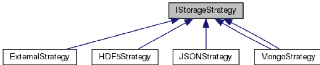
Figure 3 - Class diagram of IStorageStrategy and derivatives
