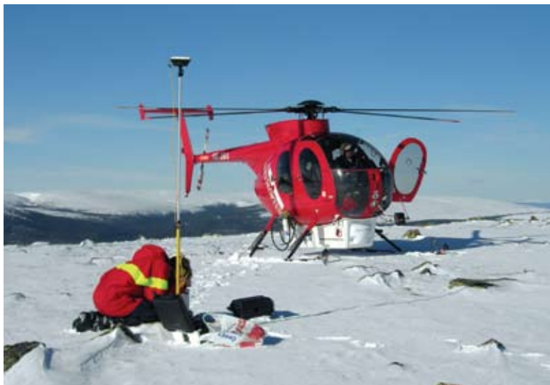
The surveys performed by the Geological Survey of Sweden include measuring the gravitational field. These data can be used to map ore-bearing formations, among other things.
