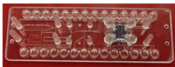
Polymer module with integrated silicon chip with silicon dioxide pillars
