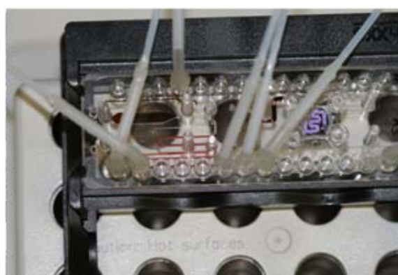
The slide with fluidic connections for sample insertion, lysis buffer and wash buffers.
