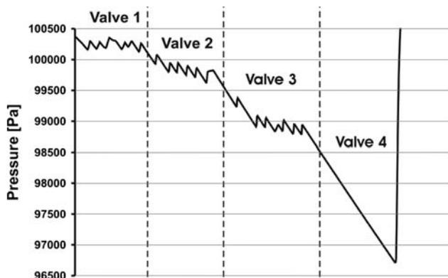
**Fig. 5** Pressure characteristics (absolute pressure) of droplet movement through the parallel actuation chip containing seven parallel channels. A constant flow rate (suction) of 10  $\mu\text{l}/\text{min}$  is applied at the common downstream end of the chip. At the fourth valve, the first droplet to break the valve effectively ventilates the system, and hence the pressure in the system returns to atmospheric conditions
