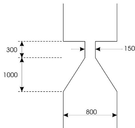
**Fig. 2** Details of capillary valve geometry (here, valve width is 150 μm). All dimensions in μm. The capillary valves contain a tapered part and a narrow restriction. The tapered part is included to aid spotting of the fluoropolymer for hydrophobization
