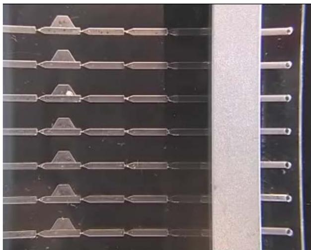
**Fig. 4** The test chip for parallel droplet movement control. Seven parallel reaction and amplification test channels are seen, each with four restrictions with hydrophobic spots. Valve pressure strength increases from right to left. In the image, 500 nl droplets are positioned before the rightmost, weakest valve
