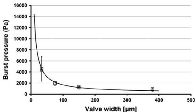
**Fig. 7** Burst pressures of the capillary valves as function of valve width. Symbols: *open square* DI water; *open circle* reagents; *solid line* represents the analytical values for water. Contact angle of DI water on Teflon was measured to be approximate 110°. The pressure data for each valve represents an average of 35 measurements (5 chips with 7 parallel channels each)
