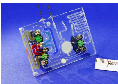
The device accepts 3 ml of sample and performs the extraction in a disposable polymer chip of credit card size. Tests performed using cancer cell lines and cervical liquid based cytology specimens confirm the extraction of HPV-mRNA by the system.
