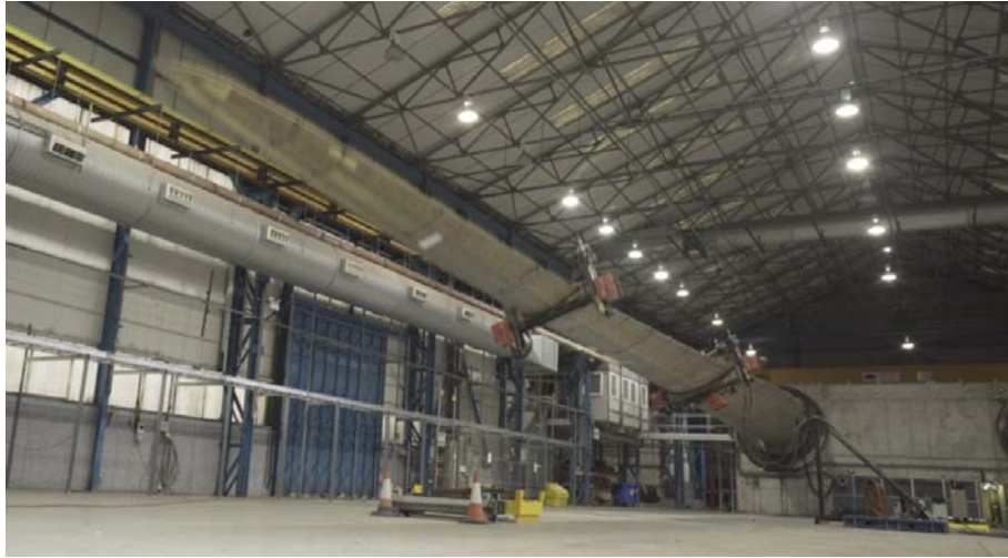
Figure 10.3 - Resonant blade fatigue testing
