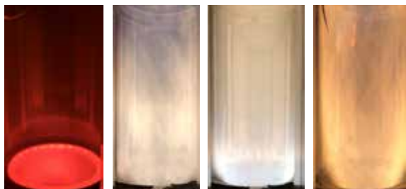
Ammonia blended flame structure in the HIPROX scaled SGT-750 burner
