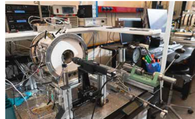
Capillary pressure, caused by interfacial tension (IFT) between reservoir fluids is the most basic rock-fluid property in multiphase flow. Image of high pressure, high temperature, pendant drop IFT measurement cell.
