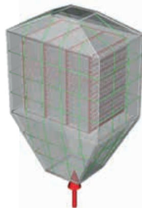
Heat recovery heat exchanger with casing and structures
