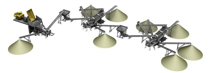
Figure 29: Portable crushing plant. Flowsheet possibilities.
