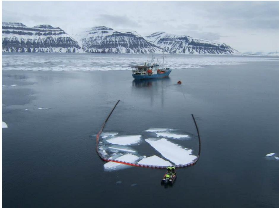
**Figure 3: AFTI boom overriding ice floes at 1.5 knots**
