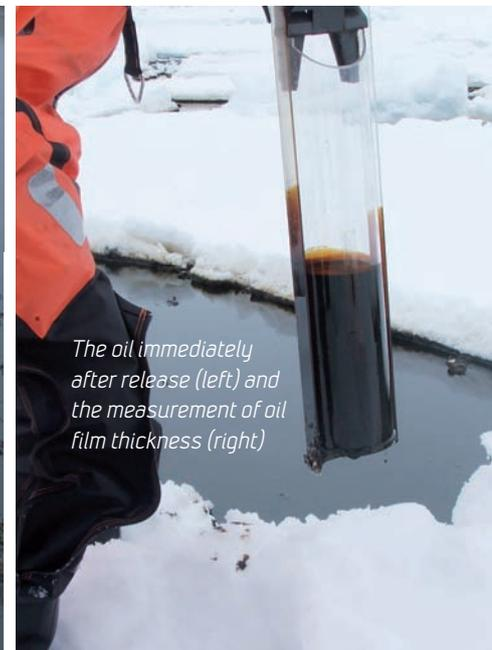
The oil immediately after release (left) and the measurement of oil film thickness (right)
