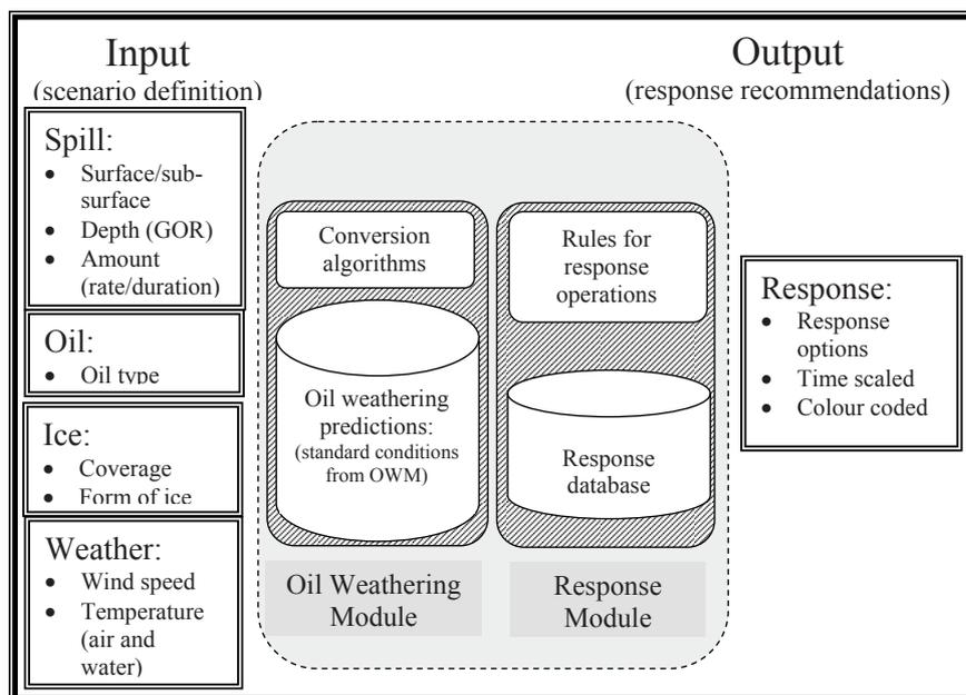
Figure 10.1 - Basic architecture of the OSRG system
