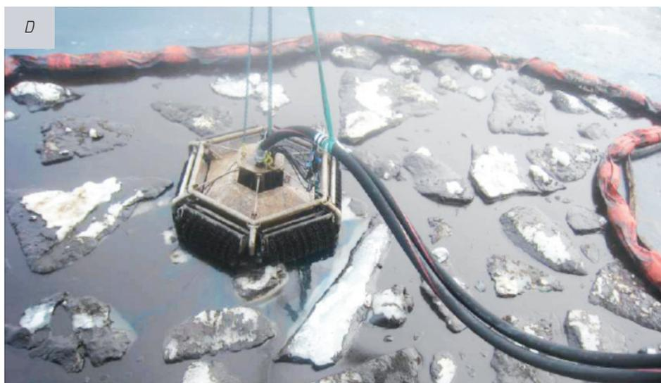
Figur 7.2 Testing of skimmers in laboratory and field experiments. A) Lamor LRB 150 Brush drum skimmer (SINTEF Sealab) B) Ro-Clean Desmi Helix (FEX 2008) C) Lamor LRB 150 Brush drum skimmer (FEX 2008) D) Ro-Clean Desmi Polar Bear (FEX 2009)
