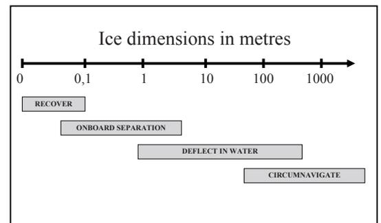
Figure 7.1 - Main ice processing principles roughly related to ice dimensions (metres)
