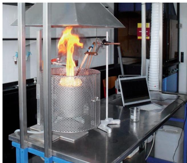
Figure 5.1 - The new laboratory burning cell during initial testing
