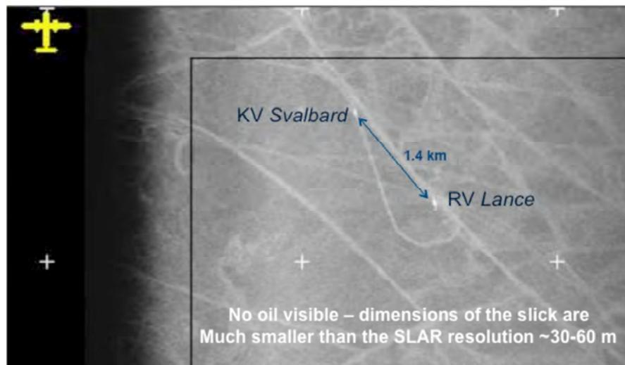
**Figure 17.** Enlarged right-hand segment from airborne SLAR imagery showing the two vessels and tracks left in the ice (within inset box). Aircraft is tracking NNW. KV *Svalbard* is slightly (~1.4 km) to the NW of *Lance*. Ice concentrations are 8 to 9+/10. Openings within the ice cover are smaller than the SLAR resolution. Source: Swedish Coast Guard
