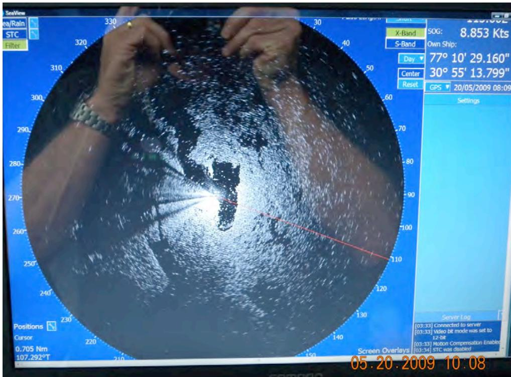
**Figure 30.** Example screen shot of Rutter Sigma S6 on KV *Svalbard*, May 20/09 clearly showing the ice around the vessel. No oil was detected.
