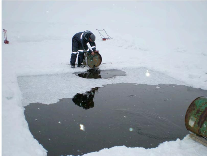
**Figure 3.** Photograph of Sintef personnel pouring oil into the spill containment area for the oil-under-snow field experiment.
