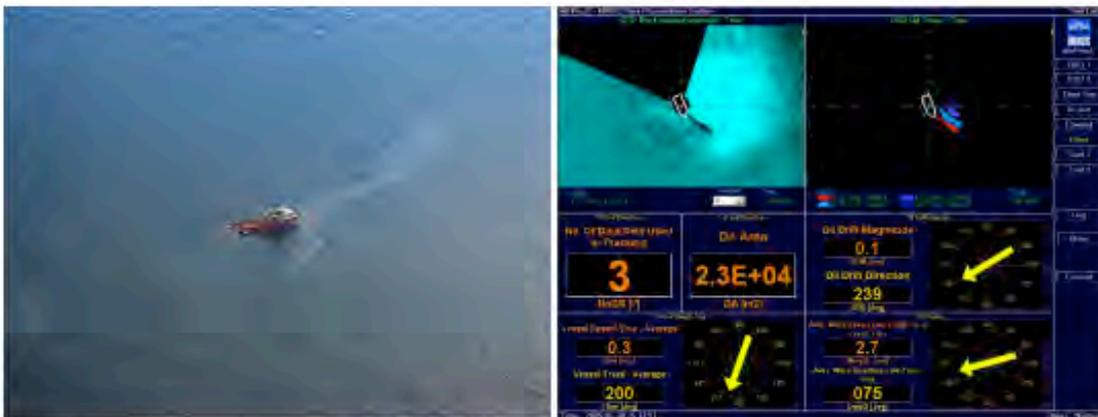
**Figure 29.** MIROS OSD, back-scatter oil oil tracking (Photo: MIROS & NOFO)
