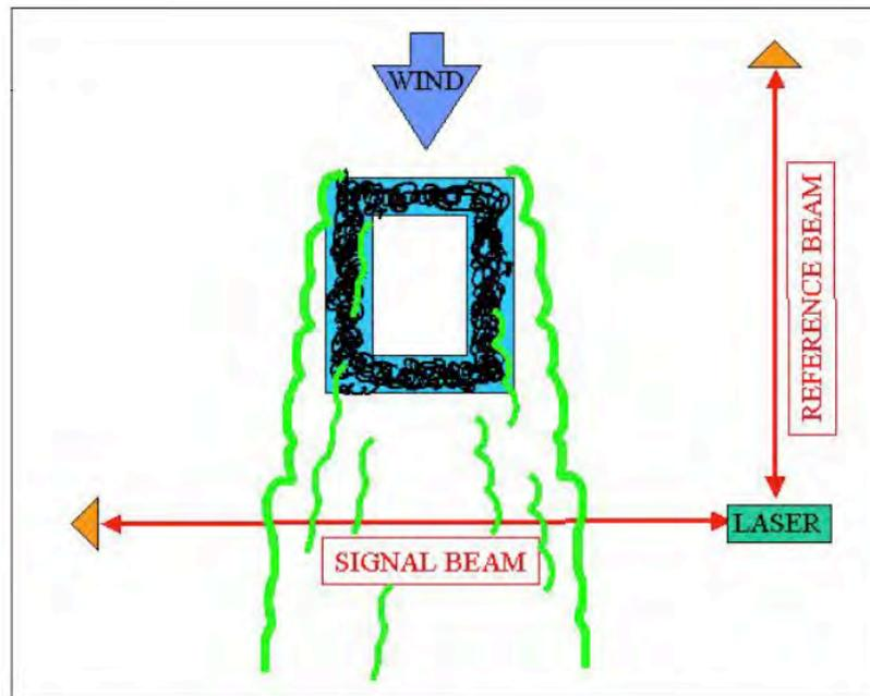
**Figure 1.** Experimental layout for the gas concentration measurements at Svea in 2007 showing the gas sensor beam orientation in relation to the circulating oil and water flume cut into the ice surface. Beam lengths were typically ~20 m operating  $\leq 10$  m downwind of the spill.
