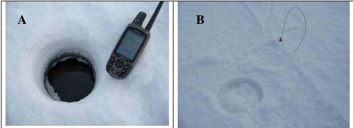
**Figure 10.** Small training oil spills used for the field training. A: 400 ml of weathered Troll crude (200°C+) in a 30cm hole in the first year ice. B: The hole is covered with snow and ice chips and marked with a small white cord.
