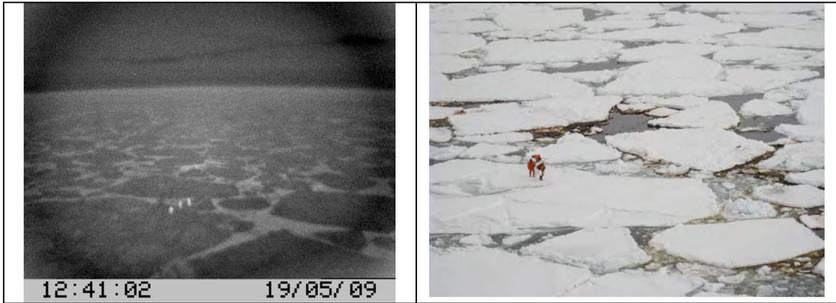
**Figure 28.** Large uncontained spill after four days at sea. Taken at daytime from the *Lance* crows nest. During daytime, the IR sensor (left) was able to distinguish between oil (white), ice-free water (light grey) and snow and clean ice floes: dark grey. Photo: Per Daling
