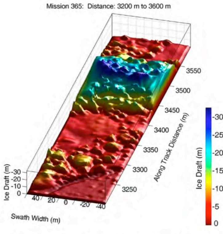
**Figure 33.** Deep 33 m ridge with shallower ridge in foreground surrounded by less deformed ice. Resolution of the mapping varies from 1-2 m. Total swath length of this mission was 23 km and up to 100 m wide. Source: Wadhams et al., 2006
