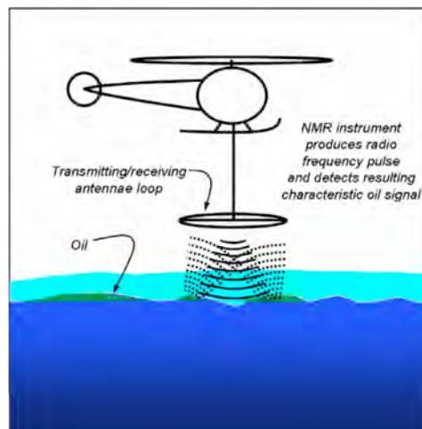
**Figure 31.** Drawing of the concept to use NMR in the Earth’s magnetic field to remotely detect oil spilled under ice. Source: Nedwed et al. (2008)
