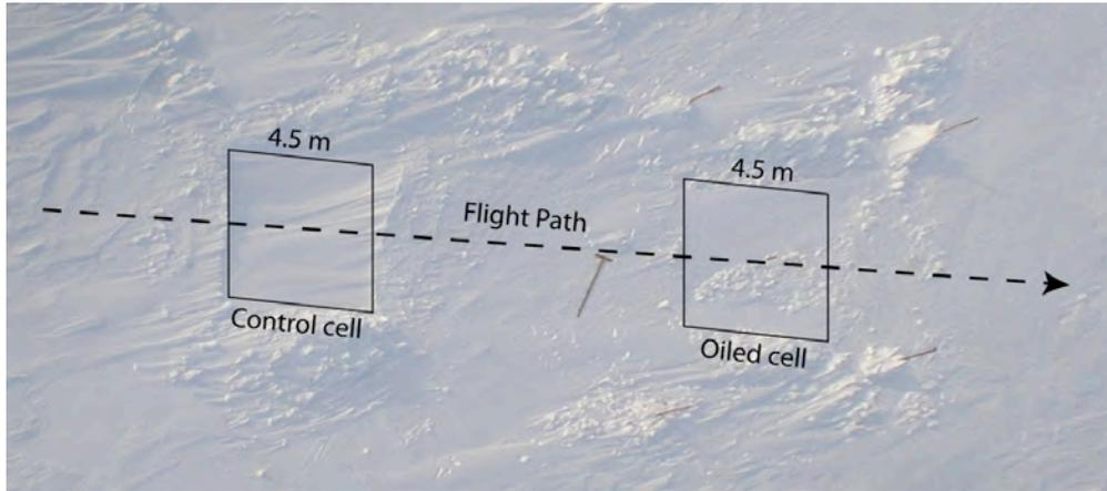
**Figure 4.** Overhead photograph of the snow covered test cells and helicopter flight path.
