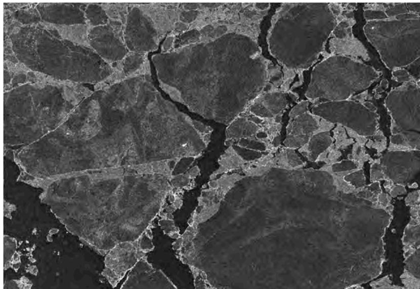
**Figure 21:** Zoom enlargement from the image shown in Fig. 20. Note the high level of detail showing rougher brash ice and smaller floes as a bright return, smoother ice areas as dark grey and open water or new ice in leads as close to black.
