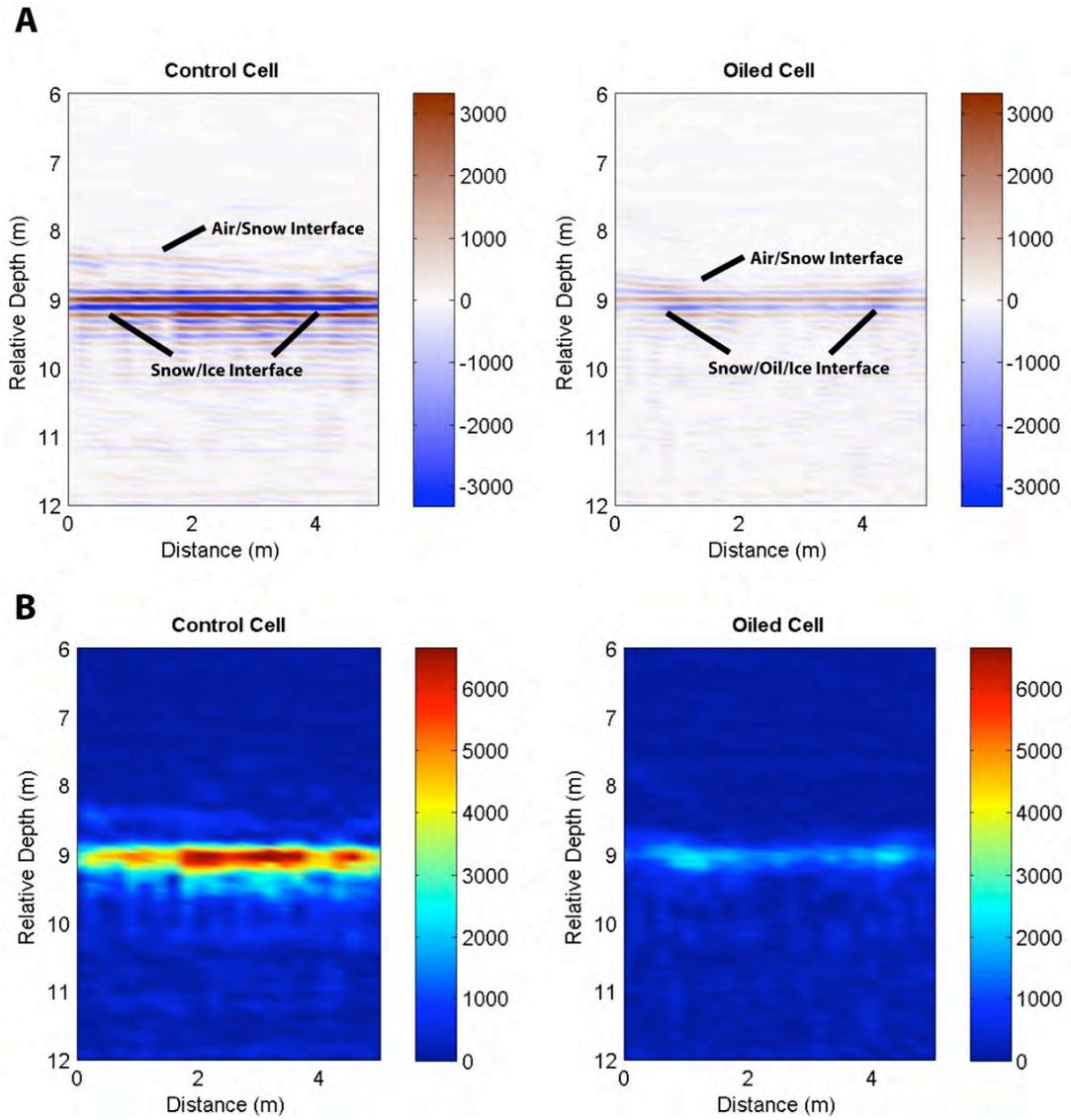
**Figure 6.** A) Plot of recorded GPR data acquired over the control and oiled cells at an altitude of 5m and speed of 2.57 m/s. B) Plot of reflection strength for the data shown in A. All data are plotted with the same amplitude scaling. Where the oil film is present, the reflection strength is reduced by ~ 45% as predicted by numerical modelling.
