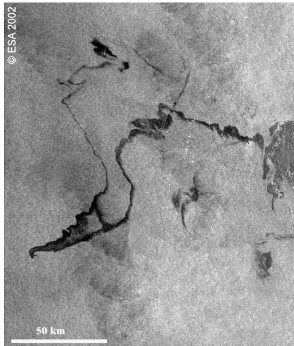
**Figure 19.** Example of previous radar satellite imagery clearly showing large slicks at sea. Envisat ASAR image (satellite) shows tanker *Prestige* 100 km off Spanish coast 20.11.2002
