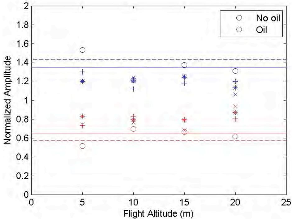
**Figure 7.** Summary of airborne radar results at speeds of 2.6 m/s (o), 5.11 m/s (+), 7.7 m/s (\*), and 10.3 m/s (x). Solid and dashed lines show the predicted amplitudes using the wind blown (low density) and undisturbed snow (high density) properties respectively. Amplitudes are normalized to the average of the clean and contaminated reflections. In all cases the amplitude of the snow-ice interface in the oiled cell is significantly lower than that in the control cell.
