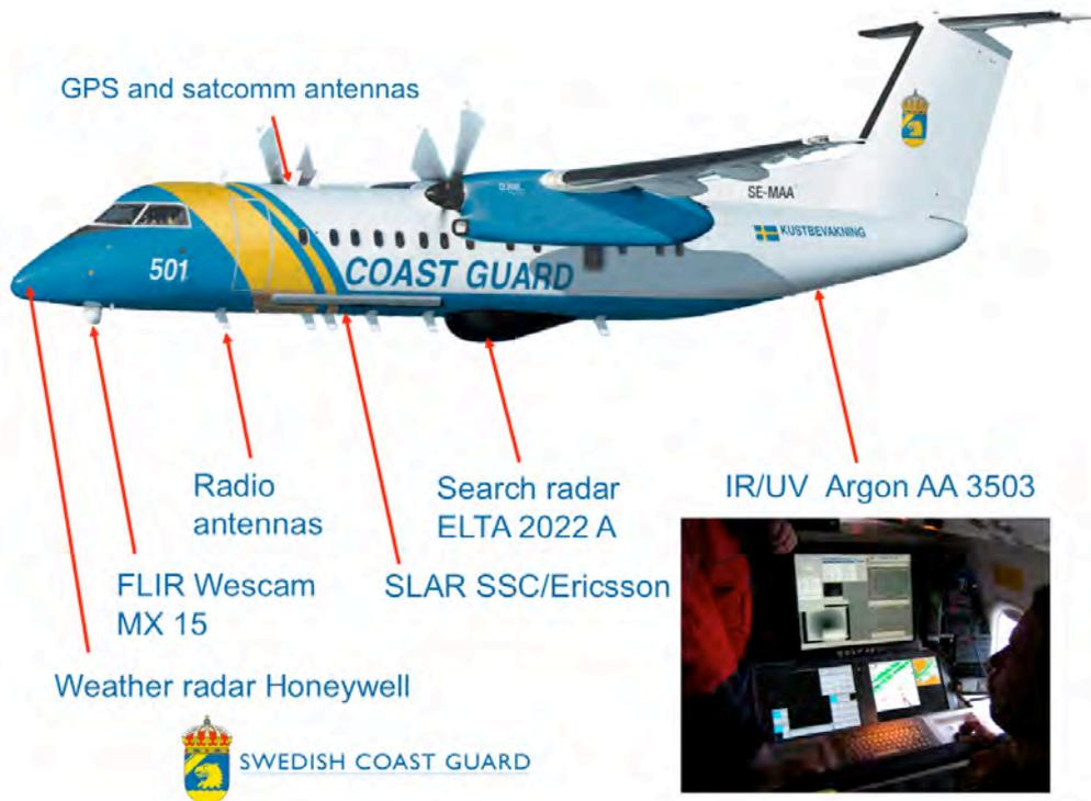
**Figure 12.** Swedish Dash 8 Q300 MSA aircraft representative of the state of the art in open water maritime pollution surveillance. Member countries of the Copenhagen, HELCOM and Bonn agreements, as well as Canada operate systems with similar capabilities. Source: Swedish Space Corporation
