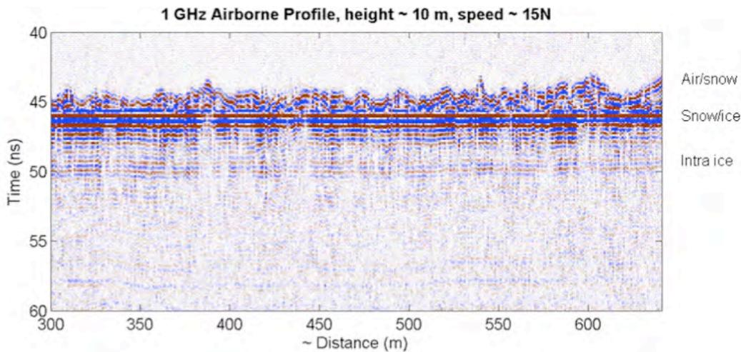
**Figure 2.** Airborne GPR profile of the snow surface on ice acquired March 2006. Radar modelling indicated that an oil layer of 1-2 cm on the ice would be detectable using commercially available GPR systems (Dickins et al. 2006/08; Bradford et al. 2010).
