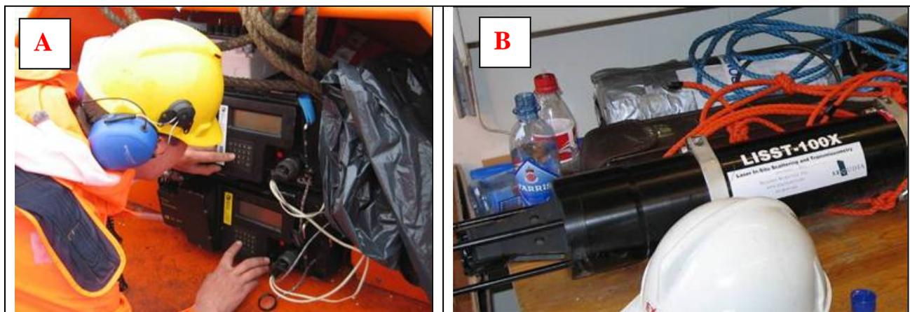
Figure 5.12 A: *In situ* UV-Fluorescence (Turner Instrument) for measuring oil concentrations in a water column. B: LISST-100X Laser diffractometer for measuring oil droplets size distribution.
