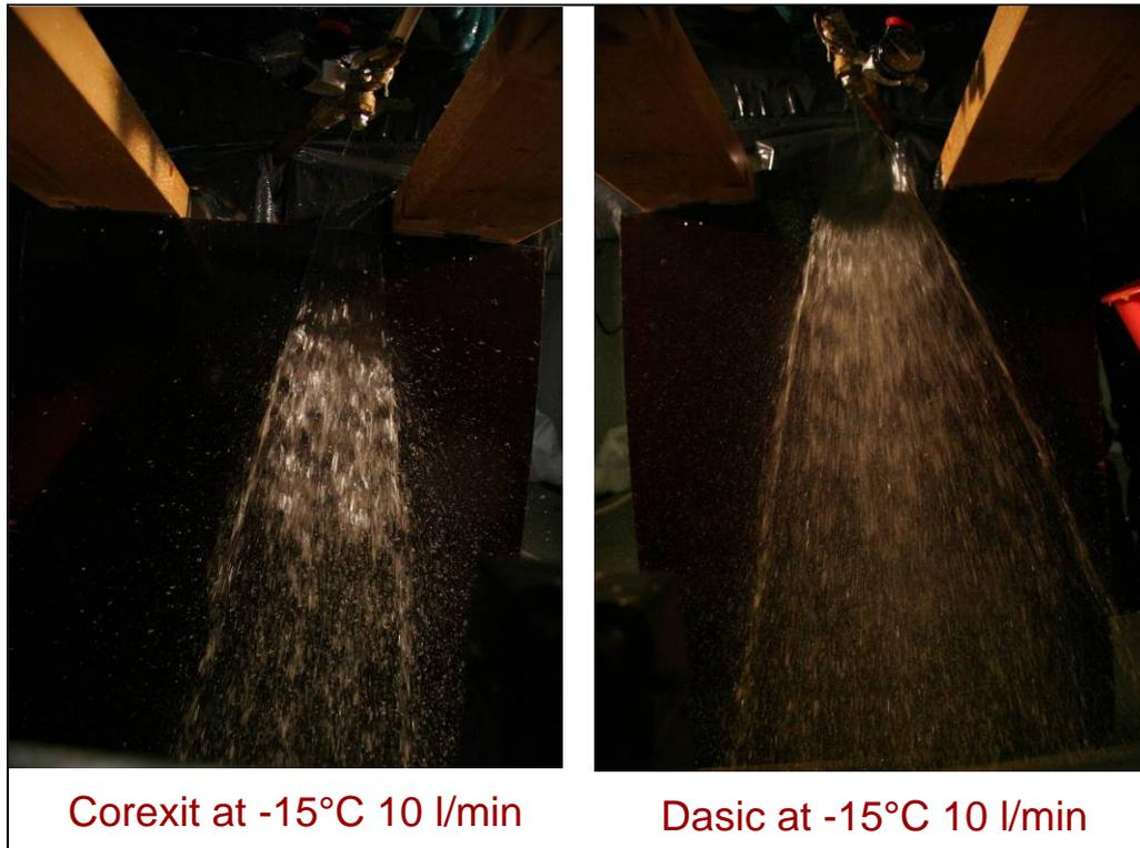
Figure 3.11 Spray pattern of Corexit 9500 and Dasic NS at  $-15^{\circ}\text{C}$ .
