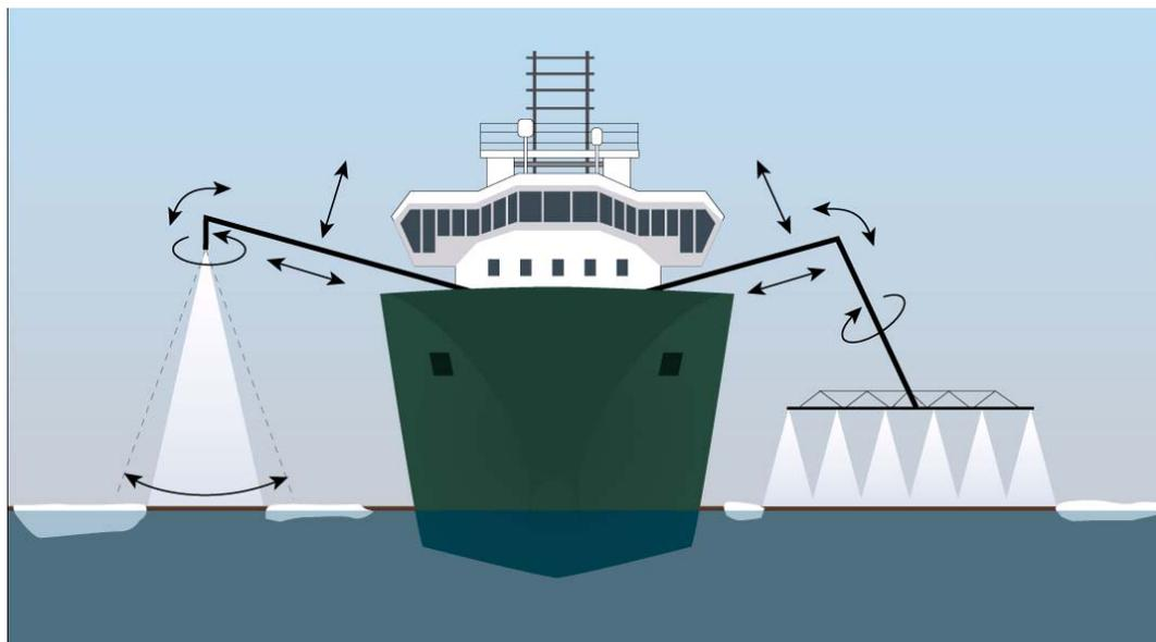
*Figure 1.2 Suggested approach for further development of a flexible spray system for use in ice-covered areas (based on preliminary thoughts at a reference group meeting in November 2006).*
