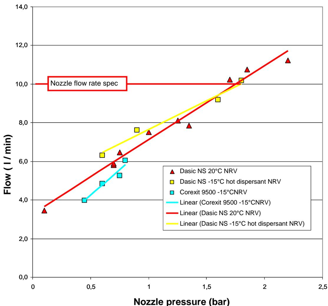
Figure 3.9 Nozzle flow rate measurements when using NRV with Dasic NS and Corexit 9500 at various test and reservoir temperatures.
