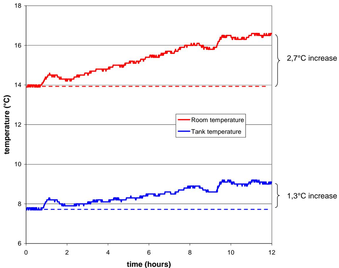
Figure 4.6 Heating of 1m<sup>3</sup> of water using floor heating. Red line: temperature in insulated day tank room; Blue line: temperature in the day tank (water).
