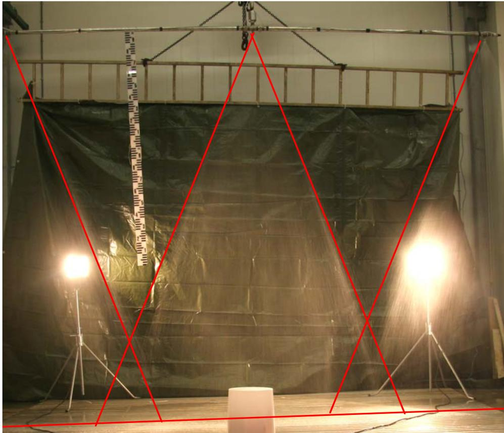
Figure 4.8 Image from the spray pattern testing. Red lines indicate an operative (average) spray angle of  $22.5^\circ$ .
