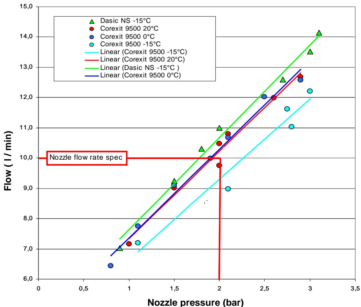
Figure 3.10 Nozzle flow rate measurements with Dasic NS and Corexit 9500 at various test temperatures (without using NRV).
