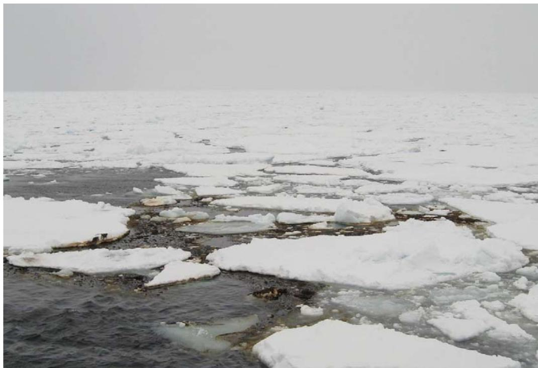
*Figure 5.5 P4.1 slick (0.5 m<sup>3</sup> of stabilized Troll B crude oil) released in 70-80% ice coverage.*
