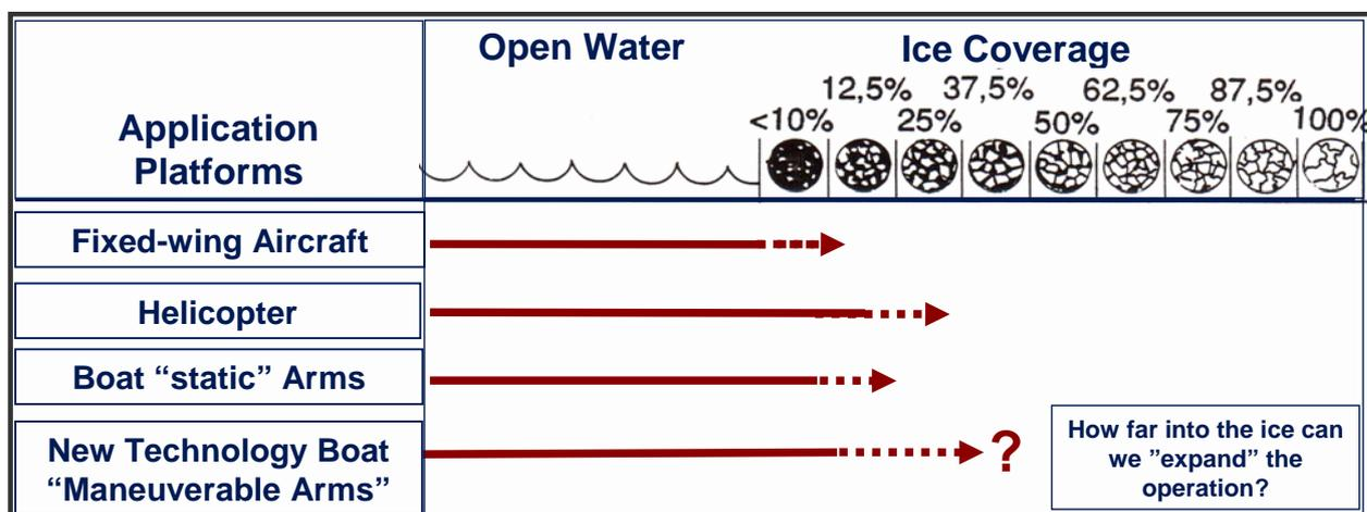
Figure 1.1 Tentative application area for various methods under different ice conditions/coverage (from a feasibility study, ONA, Daling et al., 1990).
