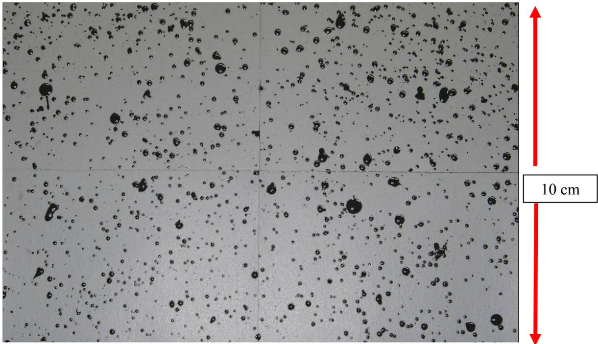
Figure 3.5 Example of oil sensitive paper exposed to a dispersant spray.
