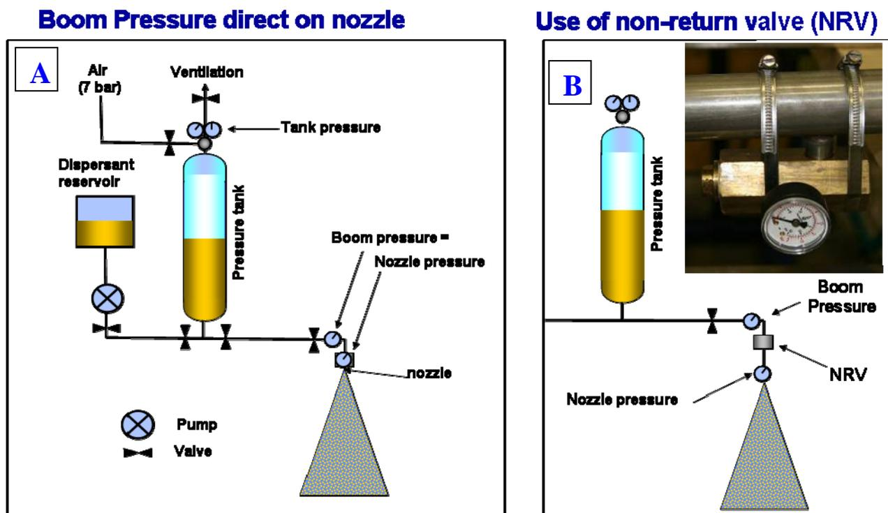
Figure 3.3 Schematic of dispersant spray rig. A: Boom pressure directly on nozzle (no NRV), B: Use of No Return Valve (NRV).
