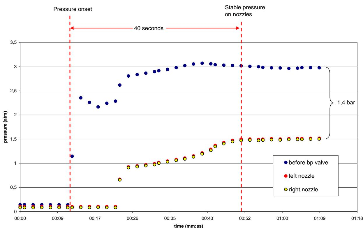
Figure 4.10 Logged pressures during the “cold start-up test.”
