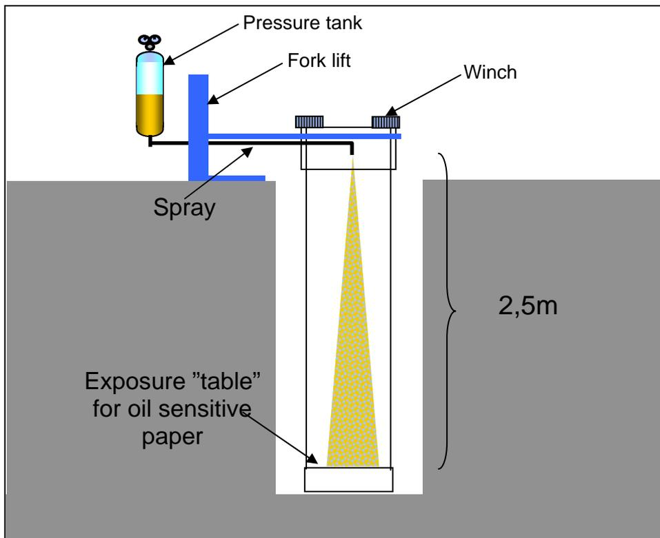
Figure 3.2 Schematic of dispersant spray rig with the 2-meter-deep basin well, with the exposure table for droplet size measurement at the well bottom.
