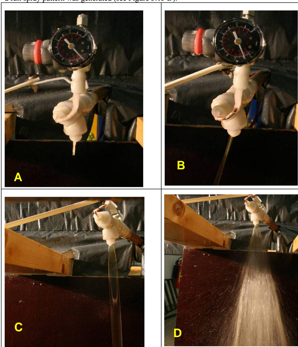
*Figure 3.13 Spray testing under freezing conditions. A: Icy nozzle after freezing at  $-15^{\circ}\text{C}$  for 24 hours just before the pump starts. B: 10 sec after starting the pump, C: 20 sec after starting the pump. D: 30 sec after starting the pump (full spray pattern).*
