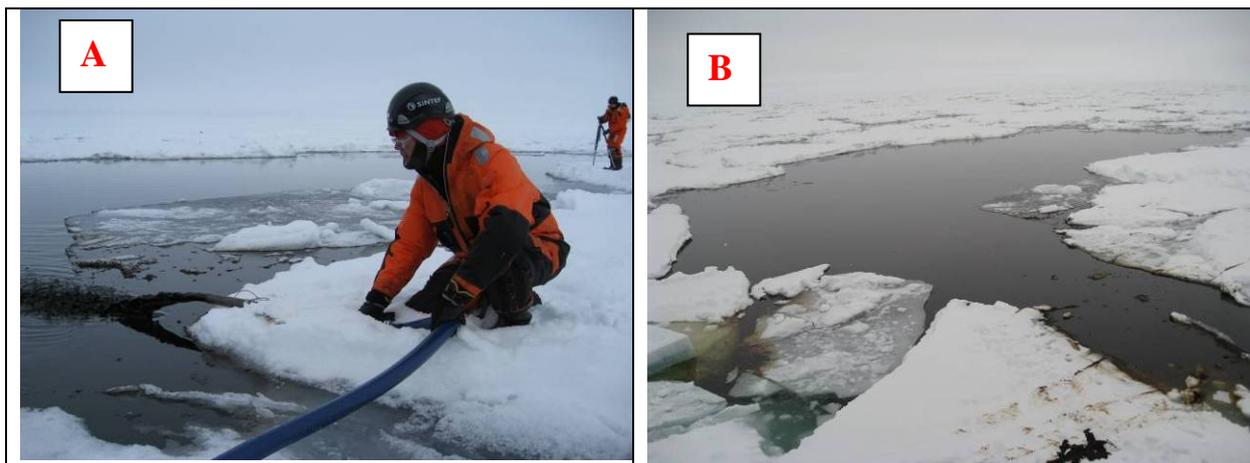
Figure 5.8 A: May 19<sup>th</sup> 09:00: Release of 2 m<sup>3</sup> of stabilized Troll B crude oil in 70-80% ice coverage from a floe about 30 m from the Lance). B: May 19<sup>th</sup> 09:15: Shape of the slick after stoppage of the release (ca. a 30m x 10 m slick).
