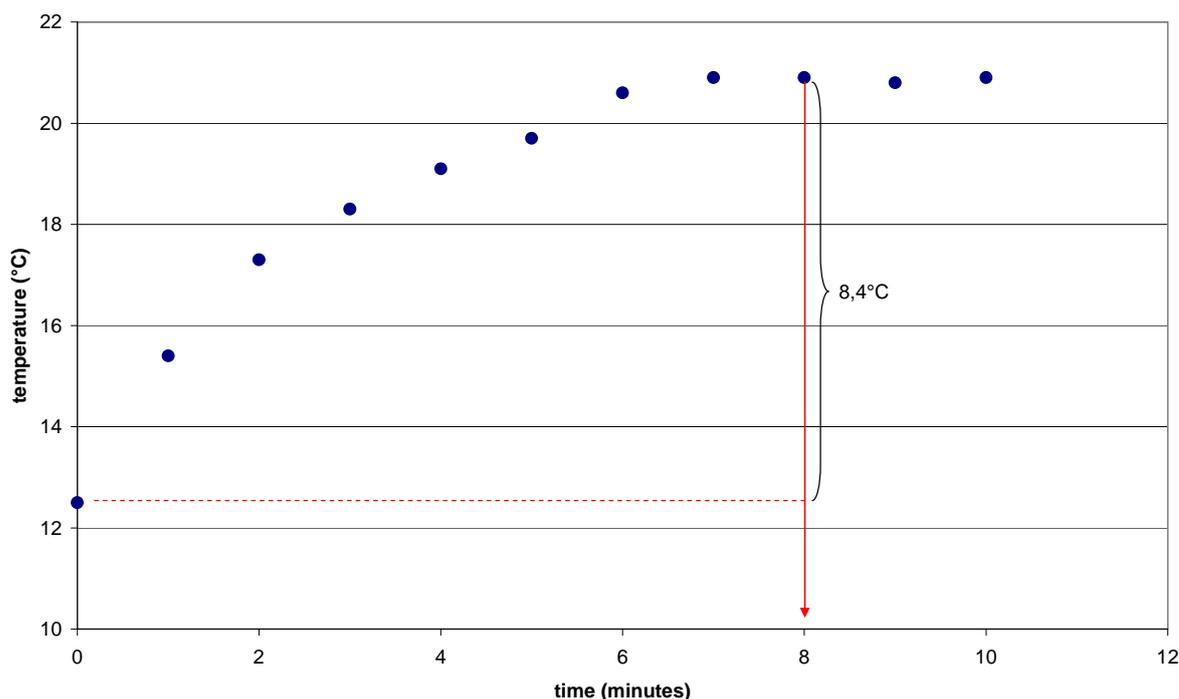
*Figure 4.7 Heating of 170 litres of dispersant using heat exchanging using hydraulic fluid.*
