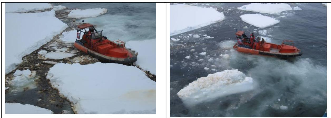
*Figure 5.14 Use of the MOB boat agitation using the water-jet of the dispersant treated oil. Left: during agitation (ca. 15-20 min after spraying). Right: Area after finishing the water jet washing.*
