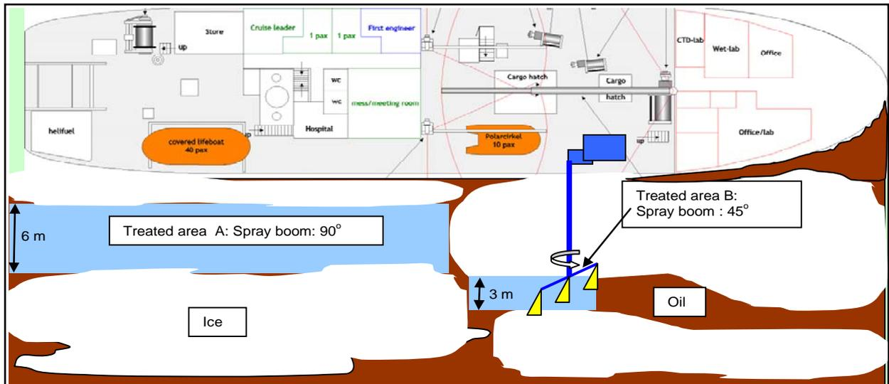
Figure 5.3 Schematic showing flexibility in adjusting the angle of the spray boom depending on the width of the oil leads.
