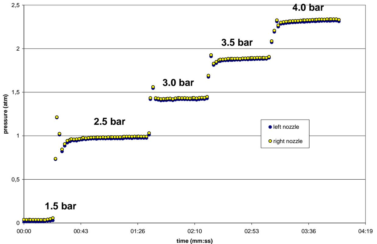
*Figure 4.5 Logged nozzle pressures during “pressure drop testing” at specific pump pressure intervals (1.5 – 4 bar) with water at 20°C.*
