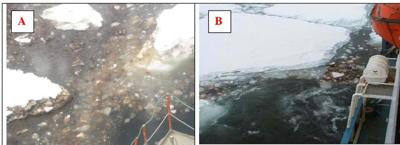
Figure 5.11 A: Details of surface oil before agitation. B: Enhancing the dispersion process by propeller wash, using the rear thrusters of the Lance 1 h after the dispersant application.
