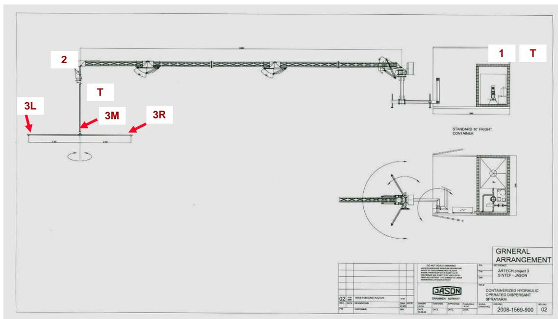
Figure 4.3 Updated technical drawing of the new application system with positions for pressure and temperature measurements.
