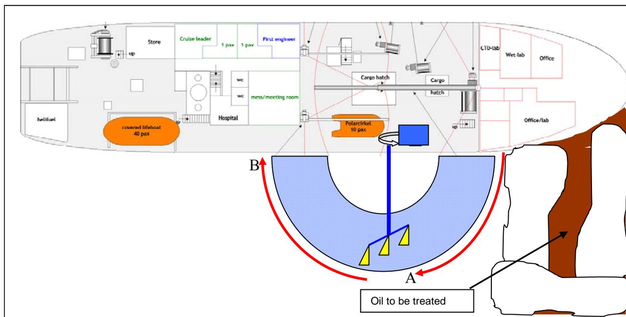
Figure 5.4 Illustration of the sweeping application area of the dispersant spray arm on the R/V Lance. A and B: Recommended horizontal rotations of the spray arm when applying on oil in leads perpendicular to the vessel's direction.
