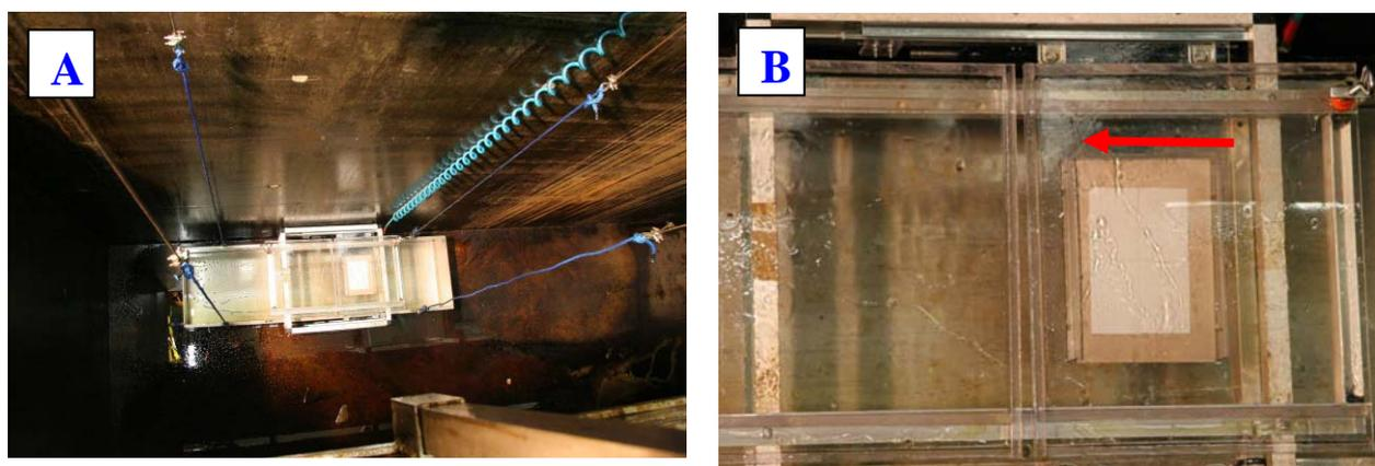
Figure 3.4 Exposure rig for dispersant droplet size distribution lowered into the 2.5 meter well.
