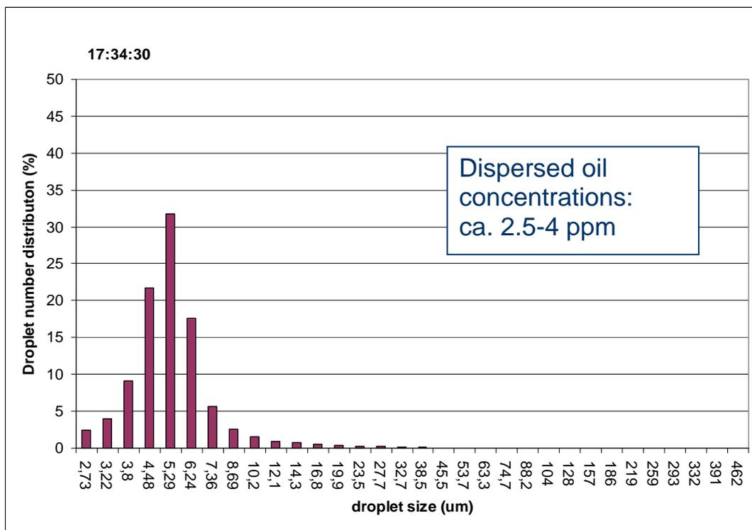
Figure 5.14 Oil droplet size distribution of dispersed oil dispersant treatment of the P4-2 slick on May 19<sup>th</sup> followed by prop washing using the thrusters on the MV Lance.
