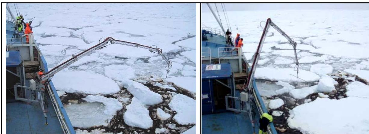
*Figure 5.6 Dispersant spraying of the 0.5 m<sup>3</sup> slick, using the new maneuverable spray hydraulic-based spray arm system.*
