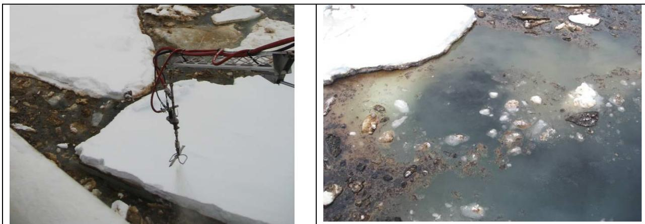
*Figure 5.13 A: Application of the P1.2 slick using a one-nozzle mouthpiece on the spray arm. B: Details of the dispersant-treated surface oil using Dasic NS before agitation.*
