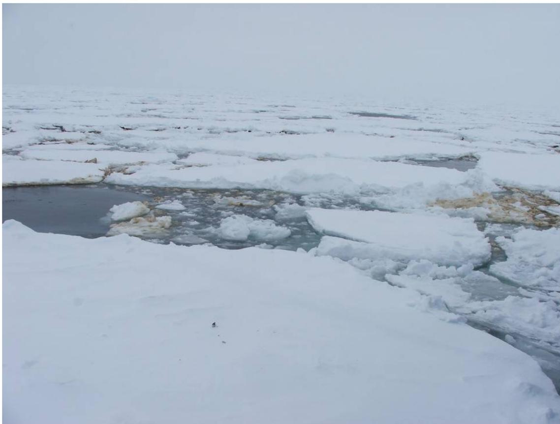
*Figure 5.7 The remainder of the P4.1 slick one day after the dispersant treatment. Only a very thin film of oil is left on the ice.*
