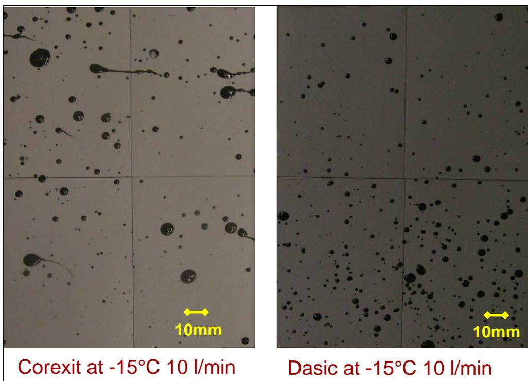
Figure 3.12 Droplet size distribution of Corexit 9500 and Dasic NS at  $-15^{\circ}\text{C}$ .
