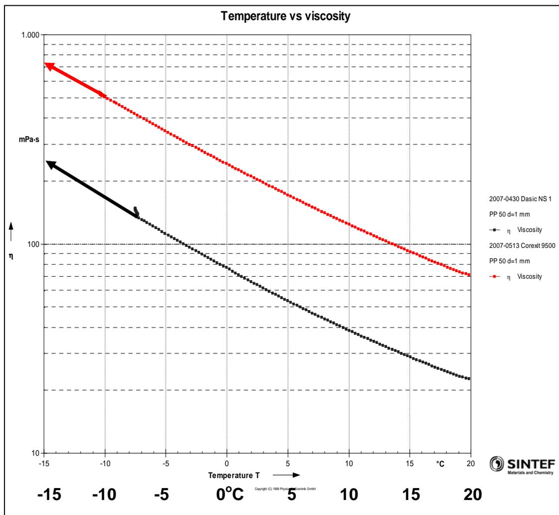
Figure 3.7 Temperature dependency of the viscosity for the dispersants, Dasic NS and Corexit 9500.
