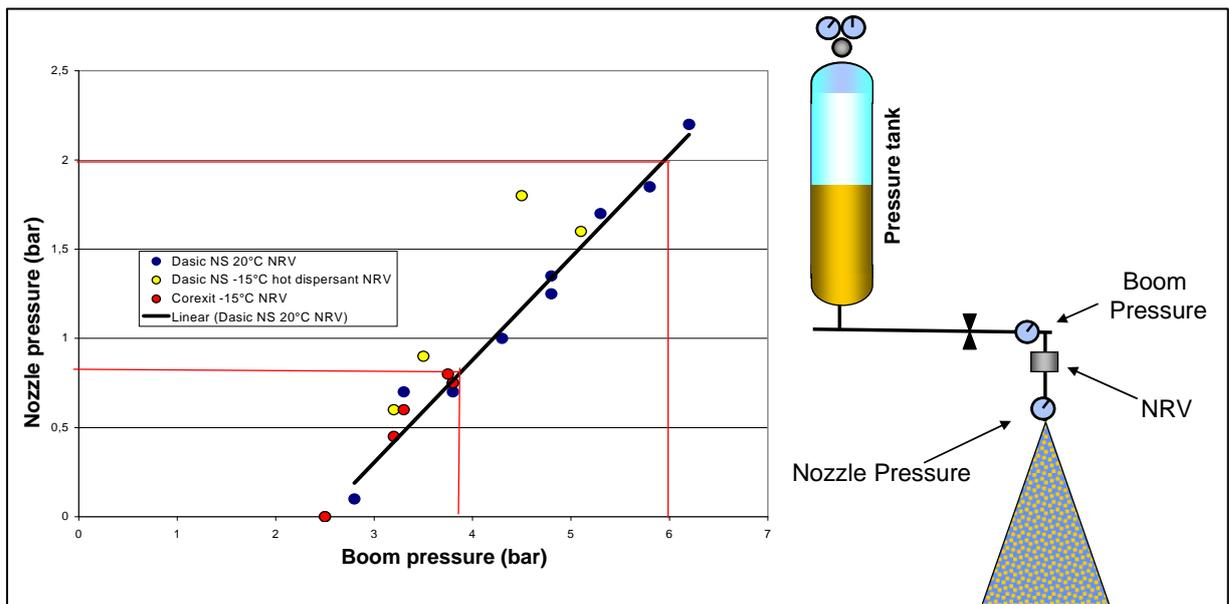
Figure 3.8 Drop in pressure in the test rig when using NRV with Dasic NS and Corexit 9500 at various test and reservoir temperatures.
