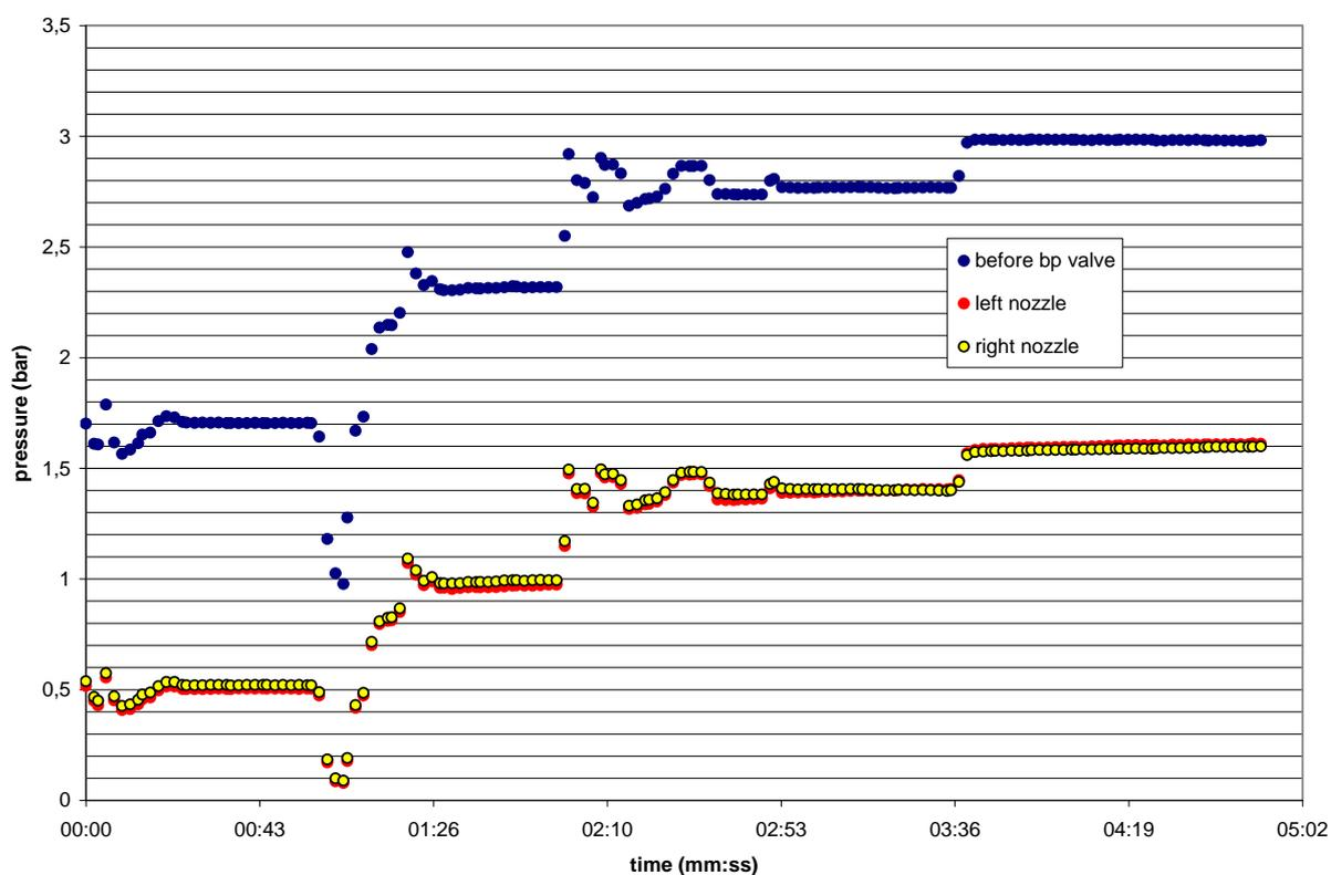
Figure 4.9 Logged nozzle pressures and pressure in front of the No Return Valve during “pressure drop testing” with dispersant at  $-5^{\circ}\text{C}$ .
