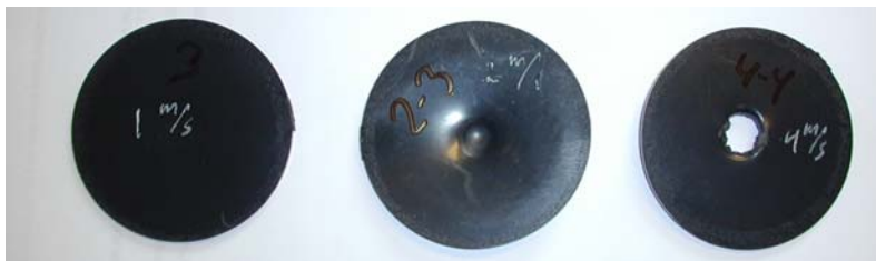
Figure 11 Deformed plates after testing with impact rates 1, 2 and 4 m/s (left to right).
