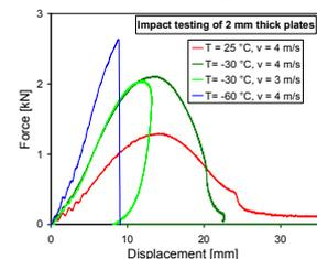
Testing of 2 mm thick plates (hemispherical  $\phi 20$  mm striker and  $\phi 40$  mm clamping ring)
