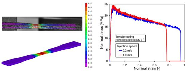
Effect of processing conditions (injection speed) on the tensile response at a rather high strain rate
