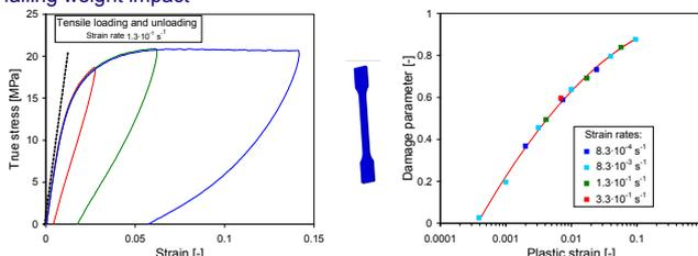
Tensile loading to different strains, followed by unloading at the same rate
