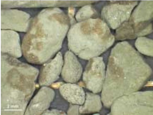
Figure 3-6 Selected shale fragments for XRD analysis from well 15/9-9, 815 m. A 2 mm scale bar is shown.
