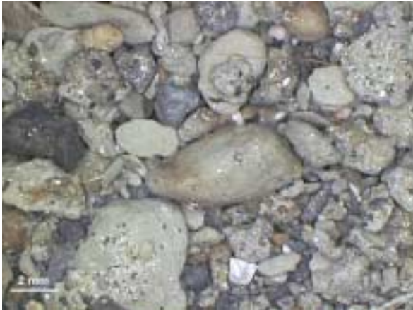
Figure 3-22 Cutting sample from well 15/9-13, 805 m. Grey shale, rock fragments, and possible dry crust. A 2 mm scale bar is shown.
