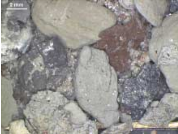
Figure 3-17 Cutting sample from well 15/9-14, 855 m, including grey shale, red shale, crystalline rock fragments and “dry crust”. A 2 mm scale bar is shown.
