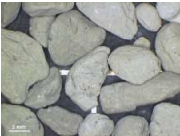
Figure 3-19 Selected fragments of grey shale for XRD analysis from well 15/9-14, 855 m. A 2 mm scale bar is shown.
