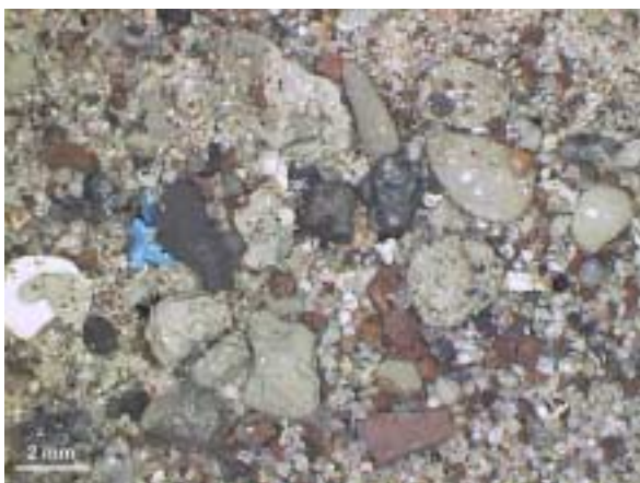
Figure 3-21 Cutting sample from well 15/9-14, 835 m. Red shale fragments occur in addition to grey. Abundant sand grains may reflect presence of sandstone in the drilled interval. A 2 mm scale bar is shown.
