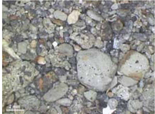
Figure 3-23 Cutting sample from well 15/9-13, 805 m. Sand-sized fragments may indicate presence of sandstone horizons. A 2 mm scale bar is shown.
