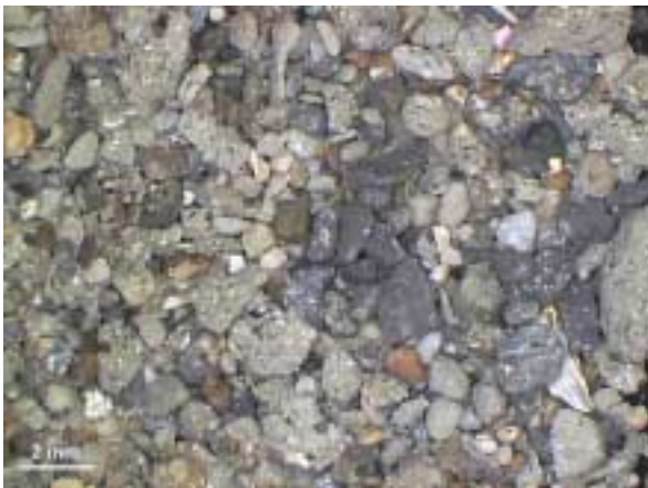
Figure 3-24 Cutting sample from well 15/9-13, 805 m. The dark grey fragments can possibly be sandstone (?). A 2 mm scale bar is shown.
