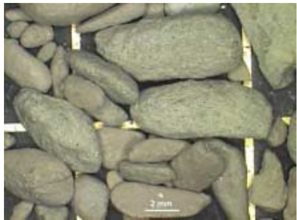
Figure 3-14 Selected shale fragments for XRD analysis from well 15/9-9, 615 m. A 2 mm scale bar is shown.
