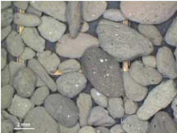
Figure 3-3 Selected shale fragments for XRD analysis from well 15/6-5, 635-645 m. A 2 mm scale bar is shown.
