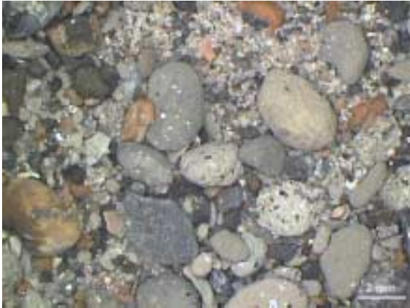
Figure 3-1 Cutting sample from well 15/6-5, 635-645 m. Abundant sand may indicate sandstone in the drilled interval. A 2 mm scale bar is shown.
