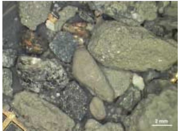
Figure 3-12 Cutting sample from well 15/9-9, 615 m. Grey shale, crystalline rock fragments, and possible sandstone fragment (left). The latter is uncertain, and it may represent concrete or dry crust of drilling mud. A 2 mm scale bar is shown.
