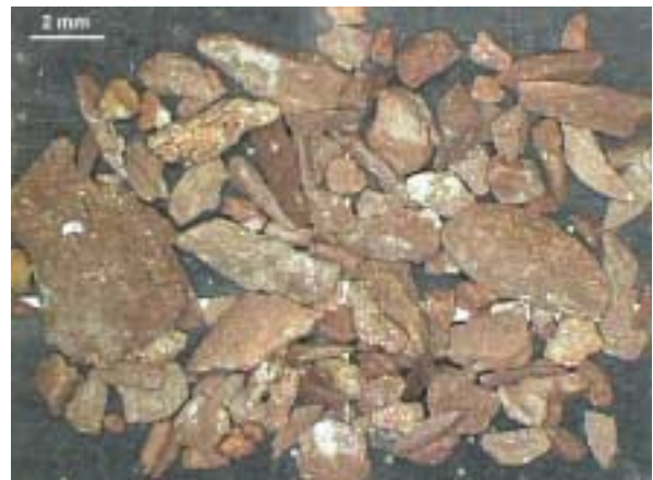
Figure 3-20 Selected red shale fragments from well 15/9-14, 855 m. A 2 mm scale bar is shown.
