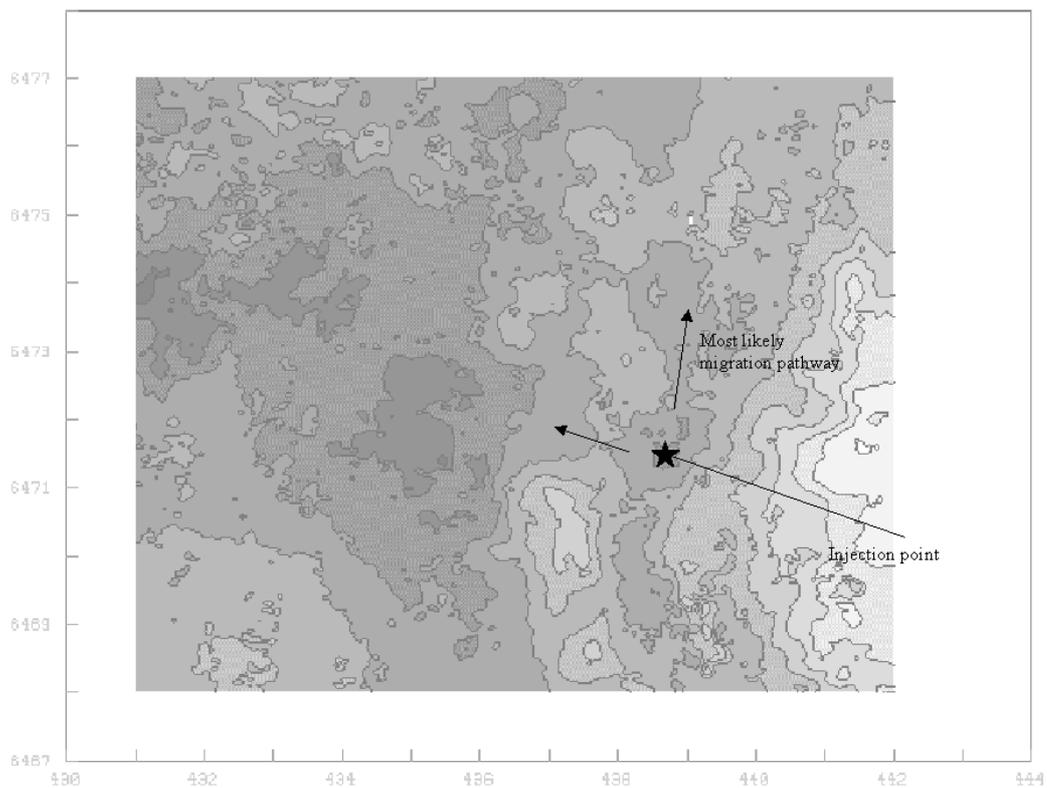
Figure 3: Depth map of the Top Utsira Sand around the injection point. The depths vary between 795 m (dark) and 900 m (light) with a contouring interval of 10 m.
