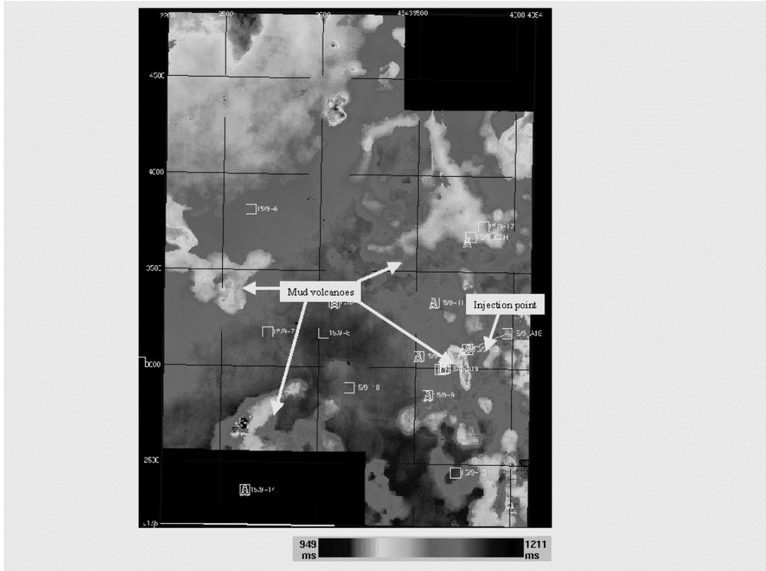
Figure 2: Map of the Base Utsira in TWT (ms) as covered by the 3D survey.
