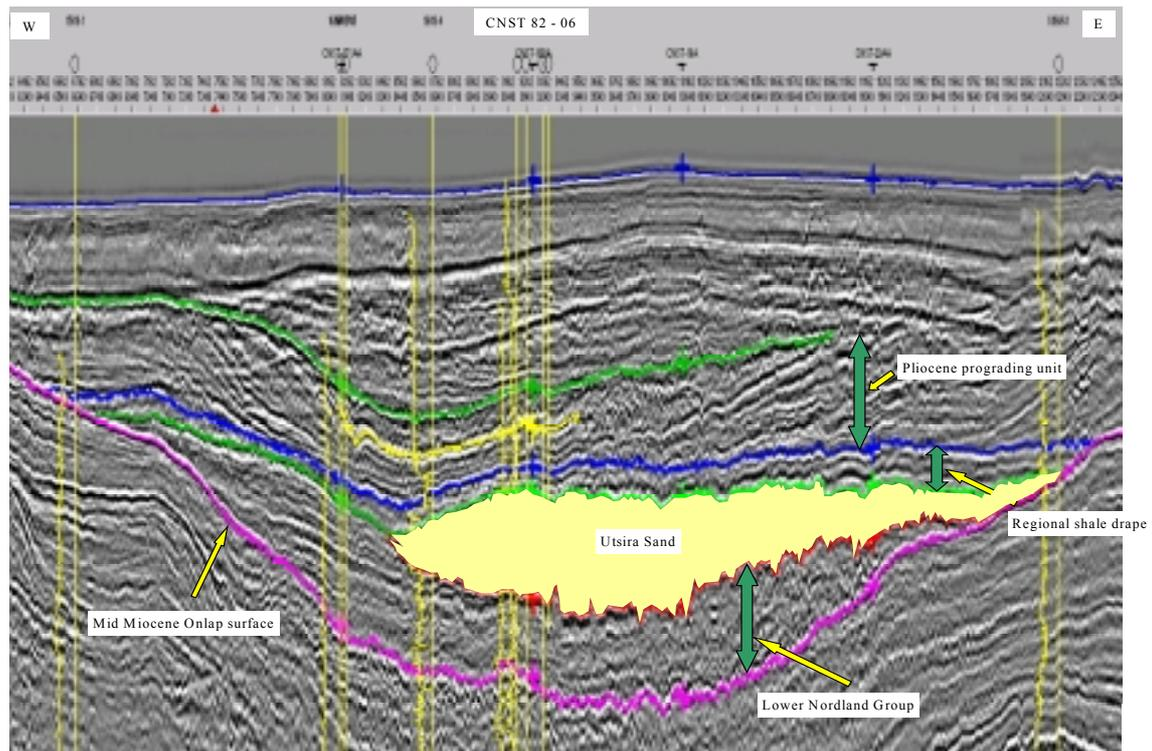
Figure 1.2 Regional seismic line through the Utsira geotechnical system
