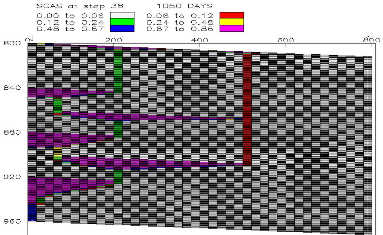
Figure 2.1 Saturation profile of the heterogeneous reservoir model at 15. August 1999. The CO<sub>2</sub> has recently reached the cap seal but large CO<sub>2</sub> bubbles have accumulated under impermeable shales.
