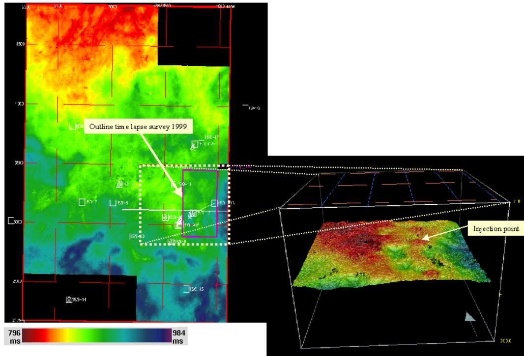
Figure 1.1 Structure map in two-way travel-time (ms) of the Top Utsira Sand around Sleipner. Note the general southerly dip and a more detailed 3D image of the Top Utsira horizon around the injection well, showing local domal and anticlinal structures. [The purple square indicates the boundaries of the 1999 time-lapse seismic survey].
