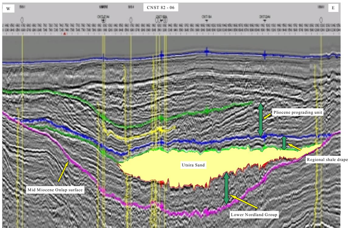
Figure 1.2 Regional seismic line through the Utsira geotechnical system
