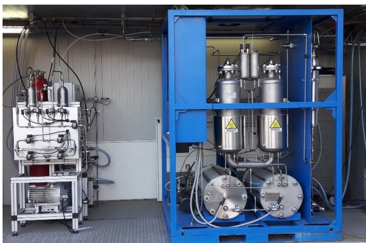
Figure 24 - Pressure swing adsorption system and alkaline electrolyser (left) - Hydrogen refilling station being used for a 350 bar refill (right)
