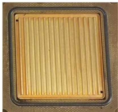
Figure1: Bipolar Plate inn a PEMWE. comparing a selection of metals and alloys under conditions similar to those inside a PEM electrolyzer.
