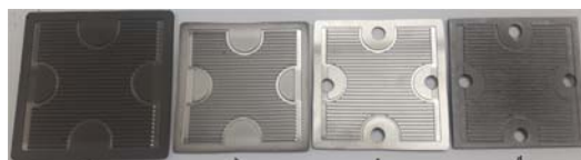
Fig 1: Image of a) pressed, b) sintered, c) machined and d) coated interconnect
