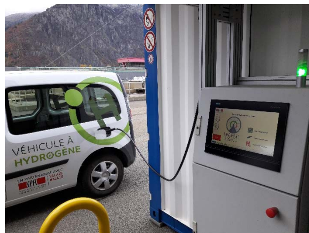
Figure 24 - Pressure swing adsorption system and alkaline electrolyser (left) - Hydrogen refilling station being used for a 350 bar refill (right)
