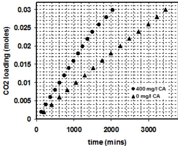
Kinetic experiments showing the rate of CO<sub>2</sub> loading in the reference (▲, 2M sodium carbonate) and catalyzed (●, 2M sodium carbonate plus 400mg/L carbonic anhydrase) tests
