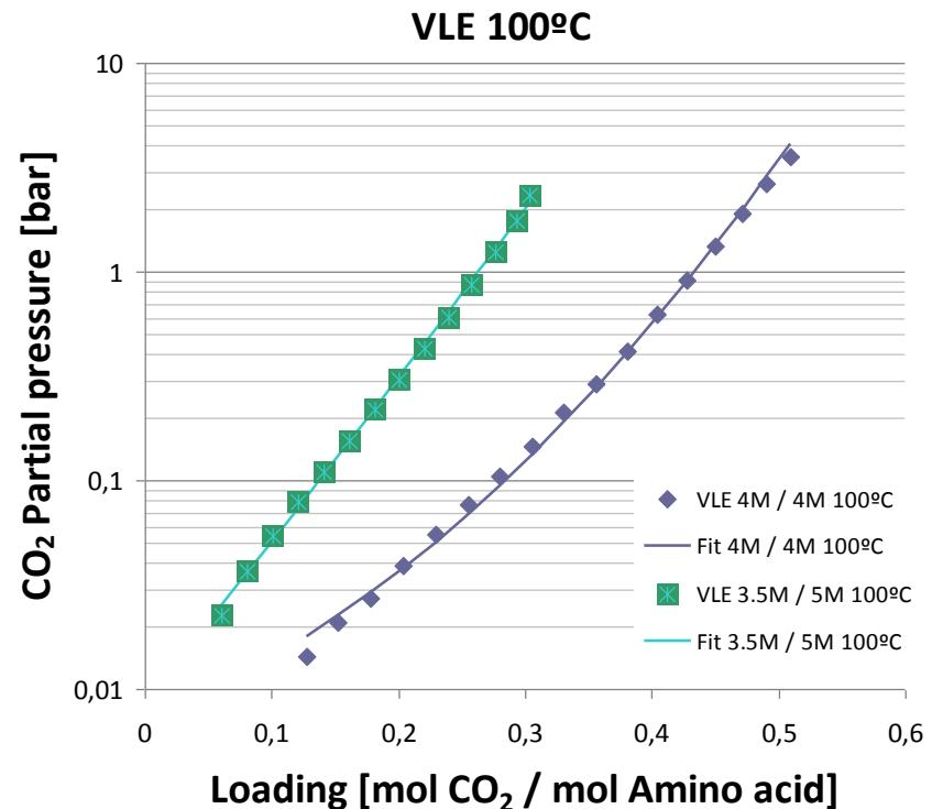
The pH shift increases the partial pressure of CO<sub>2</sub> at a given loading
