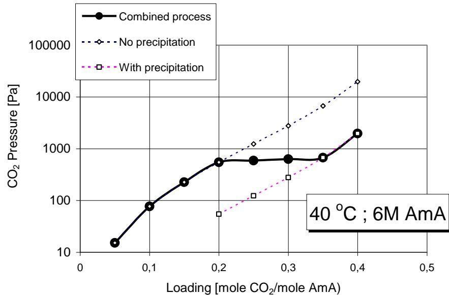
Schematic picture: effect of solvent precipitation
