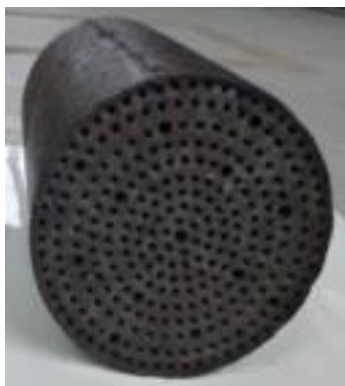
Large size adsorbent (Ø 123 mm)
