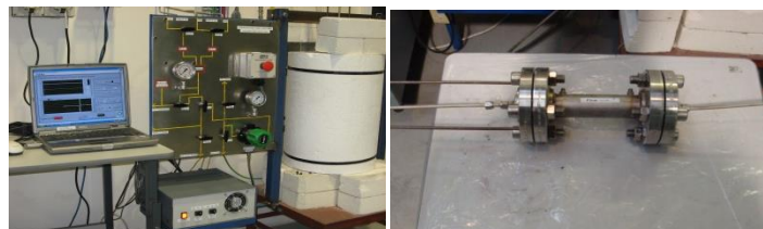
Adsorbent Characterisation Breakthrough Test Rig with Lab Scale Adsorption Chamber
