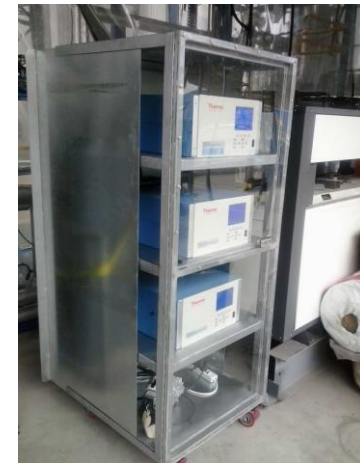
Individual sensors to measure SO x , NO x , CO and CO 2 for accurate measurement
