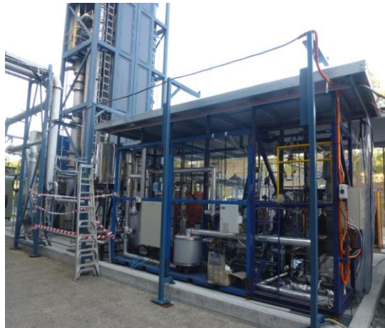
Fully commissioned solid sorbent prototype unit at Vales Point power Station
