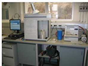
Adsorbent Characterisation Breakthrough Test Rig with Lab Scale Adsorption Chamber
