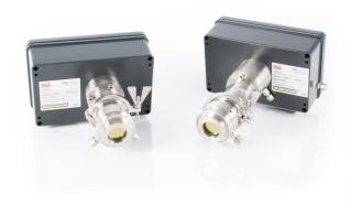
Tunable diode laser monitors are moderate cost, low maintenance instrument that sees wide-spread applications in industry. With the commercial availability of QCL lasers, applications in the mid-IR spectral range became available. The NEO LaserGas Q CF<sub>4</sub> scans over a spectral range near 1283 cm<sup>-1</sup> to record the absorbance by tetrafluoromethane CF<sub>4</sub>.
