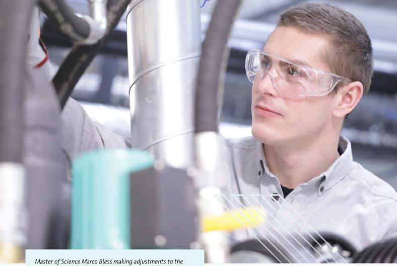
propane-butane high-temperature heat pump at HighEFFLab.
