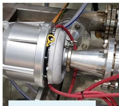
The compact high-speed turbo compressor is the key component in the steam-based hightemperature heat pump. Read more about it in the results section of Cycles – RA3, on page 46.
