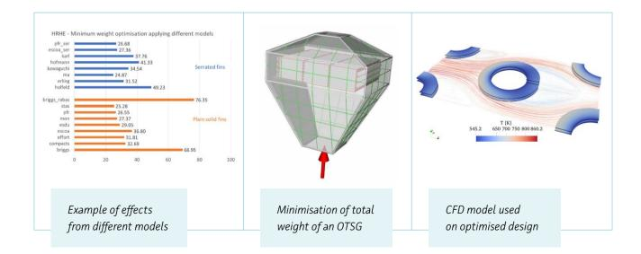
master's student's work. The work in 2022 validated the CFD model against experimental data on heatrecovery heat exchangers relevant for offshore power bottoming cycles. Effects of geometry parameters were studied. In 2023, a case study was conducted that illustrates how the choice of design models impacts minimum weight when optimising a heat recovery heat exchanger (OTSG).
