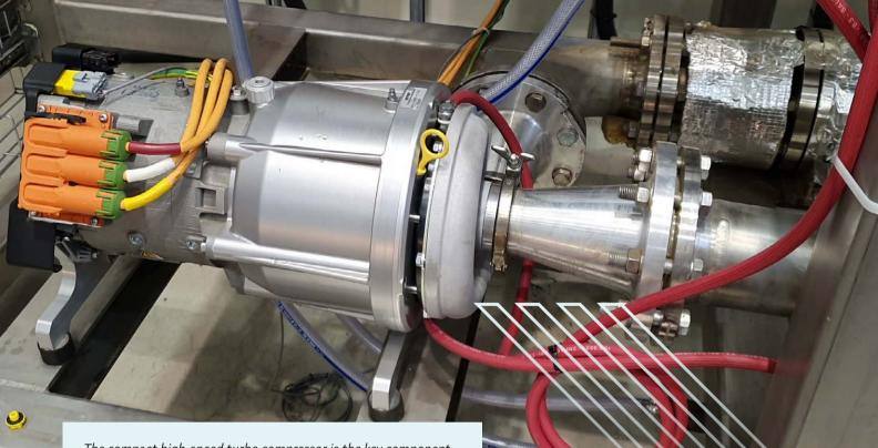
*The compact high-speed turbo compressor is the key component in the steam-based high-temperature heat pump.*
