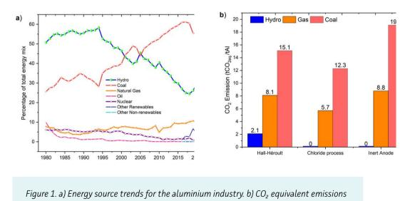
from the electrolysis process of the three technologies including the emissions from the energy sources. Data taken from International Aluminium Institute.
