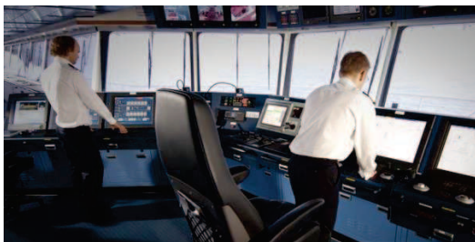
Figure 1 A modern ship bridge, here with DP-systems to the right (Kongsberg Group, 2013)
