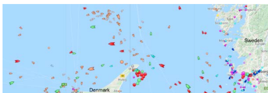
Fig. 1. This was the traffic situation at Skagen, the northern tip of Denmark at 15:00 on 5 November 2018. One may reflect on the difficulties of COLREG algorithms needed to do collision avoidance in such an area where giving way to one ship might lead into another conflict situation in an unpredictable, cascading manner (screen shot from MarineTraffic.com).
