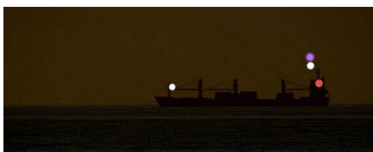
Fig.2: Should ships navigating in autonomous mode carry a special identification light? The behavior of the navigation AI maybe different from the behavior of normal, manned ships. The light could be purple which is a color that is not used for other purposes. The same discussion and color choice is debated in the autonomous car industry.
